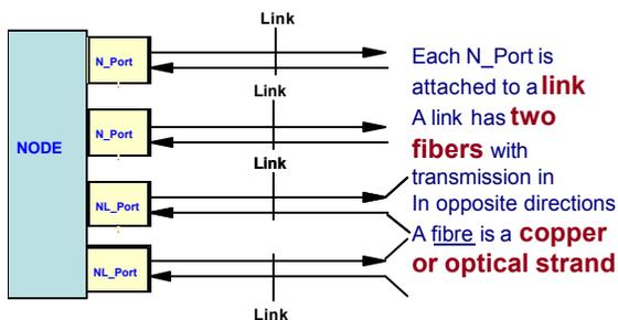
You may notice that the figure also illustrates that a single physical Fibre Channel link is comprised of two independent fibers: a dedicated transmit and a dedicated receive. This means that the port is full-duplex capable of receiving and transmitting concurrently. In fact, in a switched topology a port can be receiving data from a source port while
