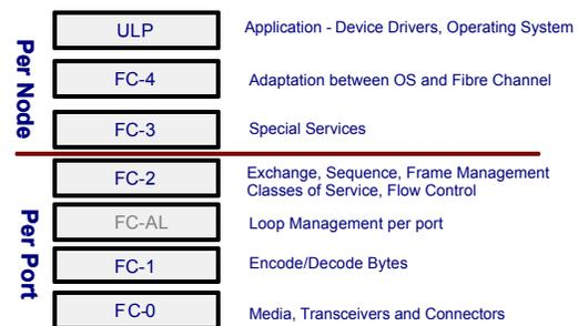
FC-0, the bottom level, describes the Physical Interface for Fibre Channel. This level specifically defines the speeds, transceivers, connectors, and cabling. Currently there are three baud rates shipping in commercial and military avionics Fibre Channel products. These are 1.0625 gigabaud, 2.125 gigabaud, and 4.25 gigabaud. These rates translate to duplex user data rates of 200 Megabytes per second, 400 Megabytes per second, and 800 Megabytes per second respectively.
