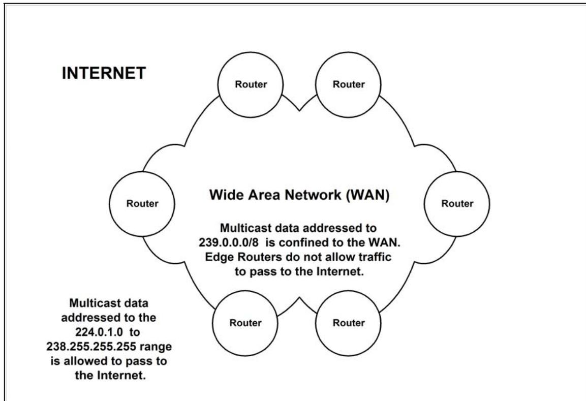
**Figure D – Scope of Multicast IP Ranges**
