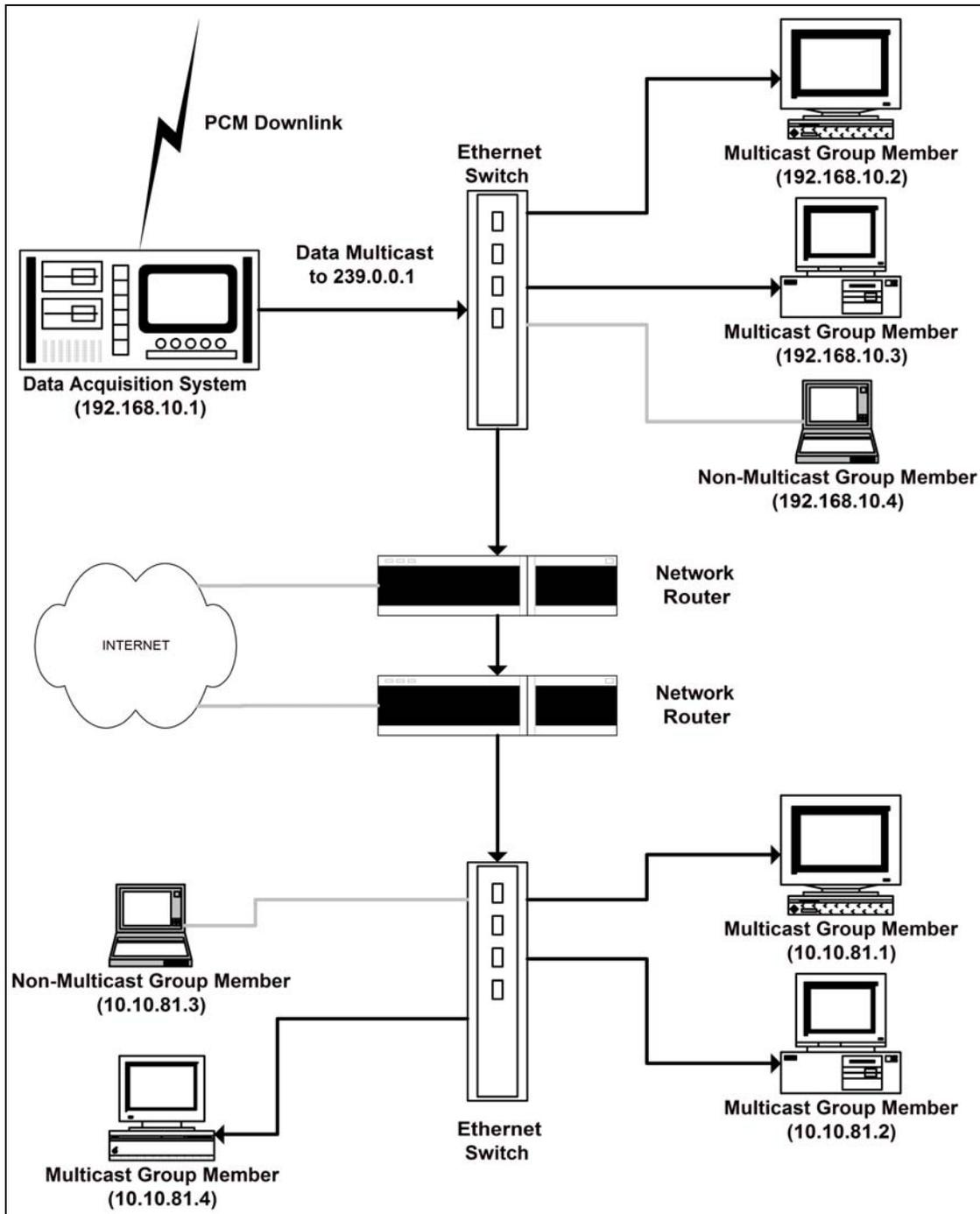
**Figure E – Single PCM Stream Multicast Distribution Design**
