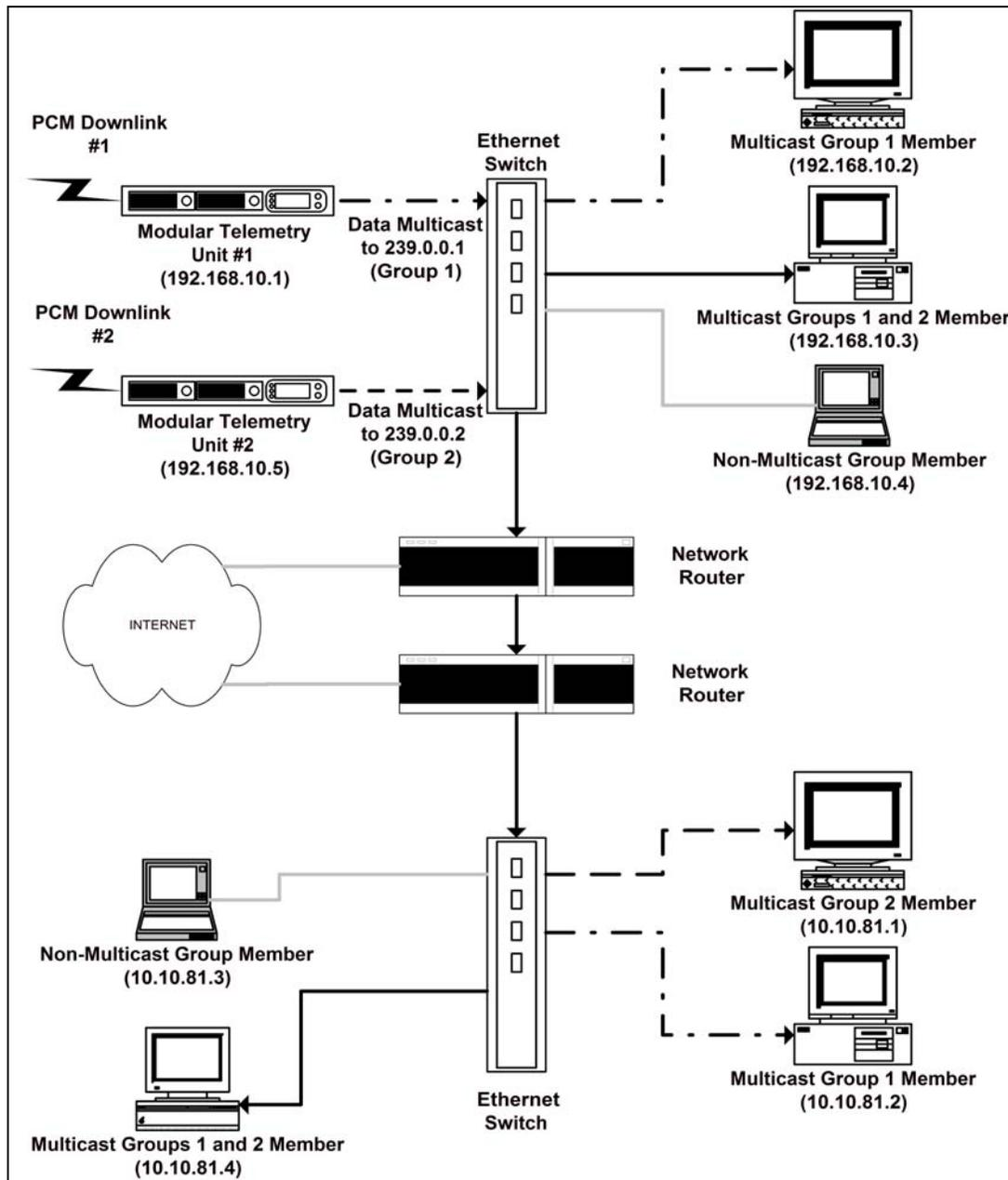
**Figure G: Multi-source Multiple Multicast Address Implementation**
