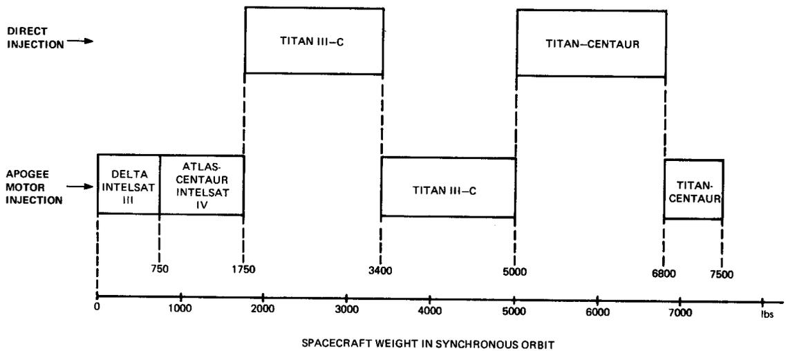
**FIGURE 3 LAUNCH VEHICLES AND INJECTION METHODS**
