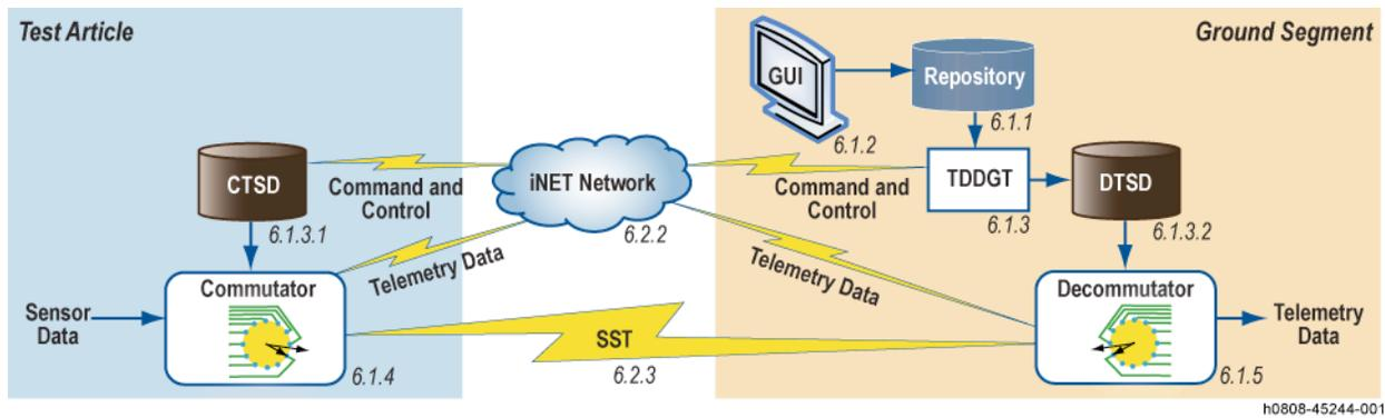
**Figure 1. The DCDS Architecture Supports Enhanced Tools to Define and Optimize the Telemetry Stream**
