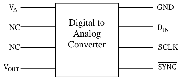
Fig.4 Pin Configuration of DAC
