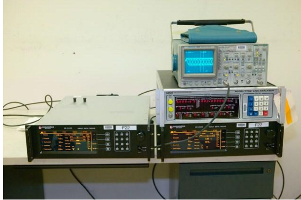
Figure 6. BER Test Equipment Setup.
