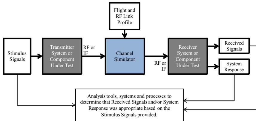
Figure 3. Use of Channel Simulators to test Receivers and Transmitters as a system.
