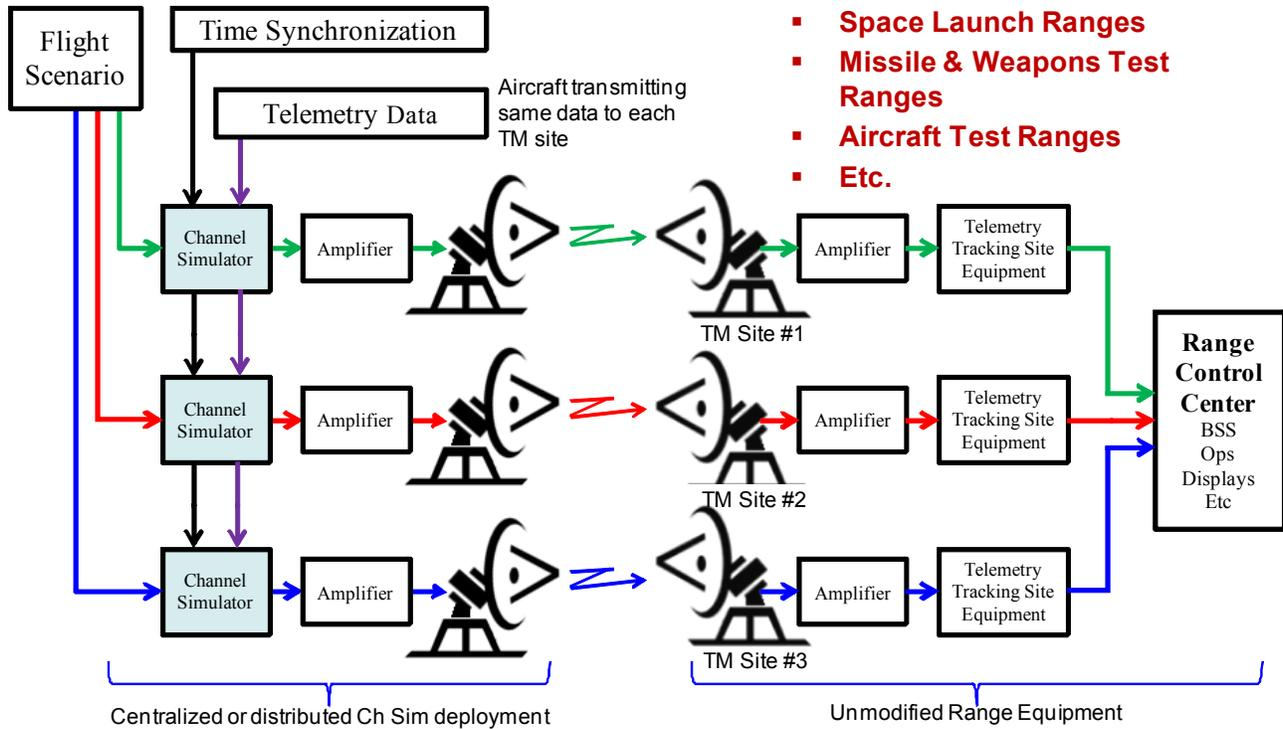
Figure 12. RTS configured to simulate 3 TM Sites simultaneously.
