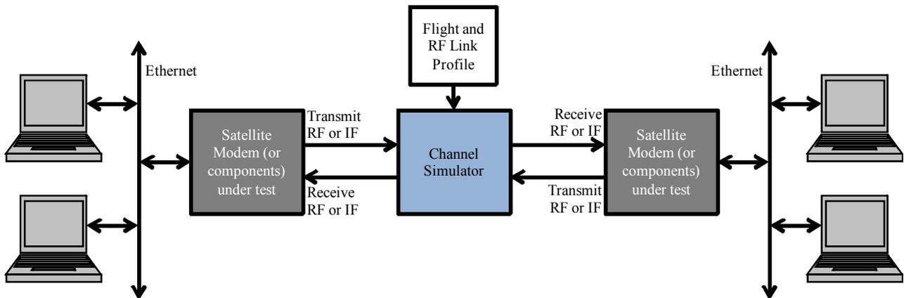
Figure 4. Typical Channel Simulator application to test Satellite ACM Modems.
