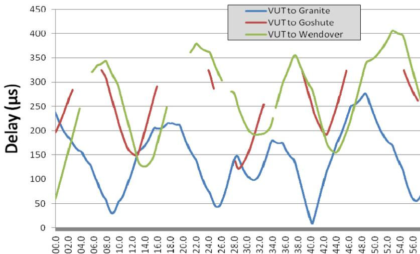
Figure 9. Elapsed flight time vs. range delay between the flight vehicle and 3 TM Sites.
