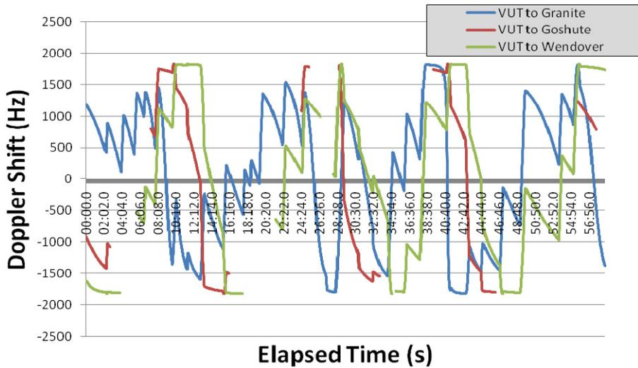
Figure 11. Elapsed flight time vs. Doppler shift between the flight vehicle and 3 TM Sites.
