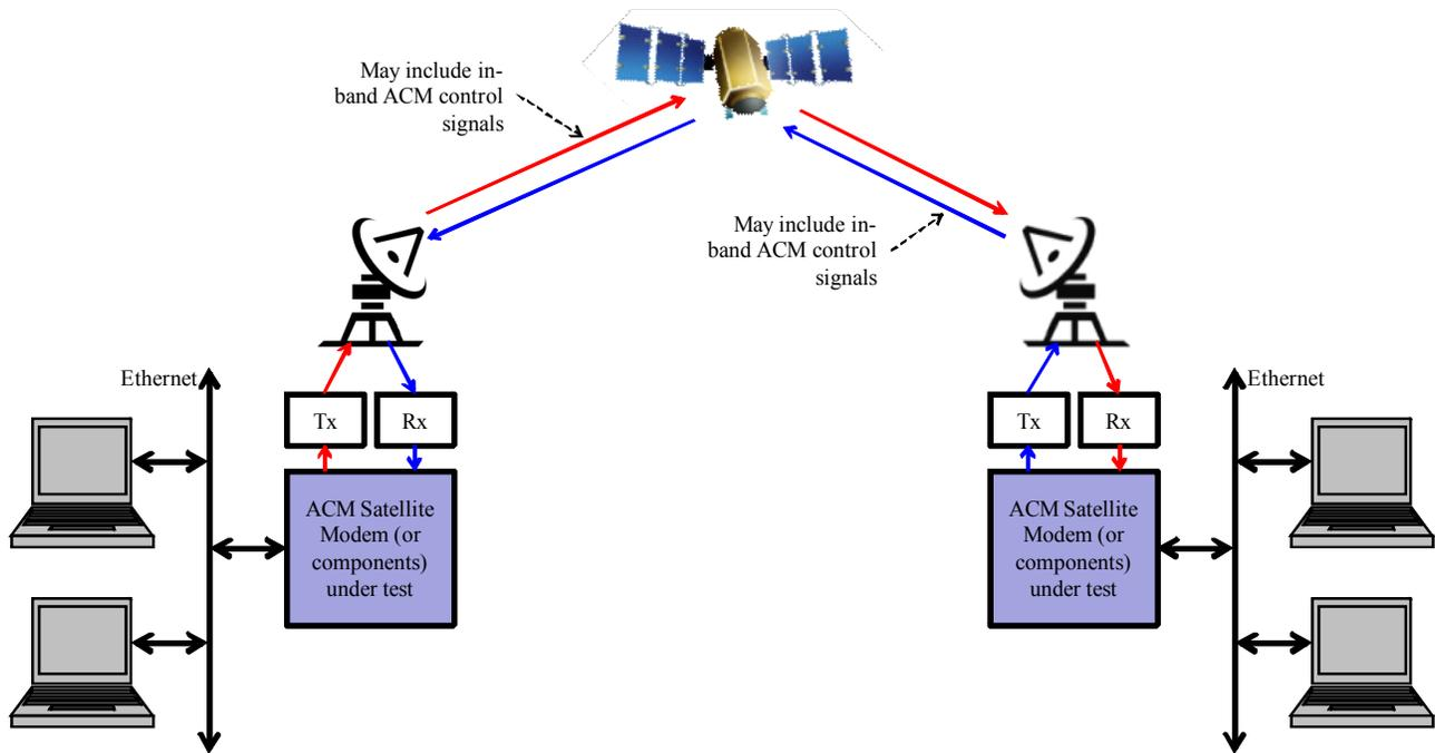
Figure 5. Example operational scheme for Satellite ACM Modems.
