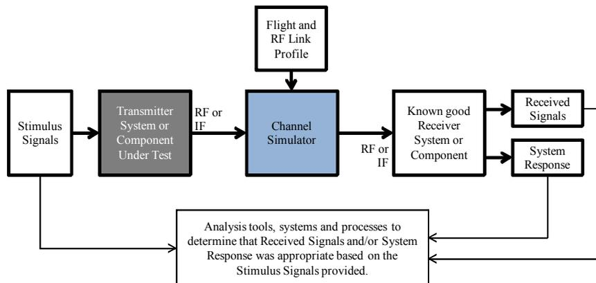
Figure 2. Use of Channel Simulators to test Transmitter Systems.
