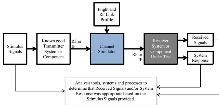
Figure 1. Use of Channel Simulators to test Receiver Systems.
