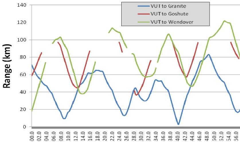
Figure 8. Elapsed flight time vs. range between flight vehicle and 3 TM Sites.
