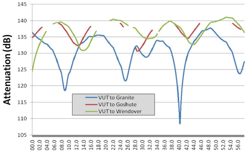
Figure 10. Elapsed flight time vs. path loss between the flight vehicle and 3 TM Sites.
