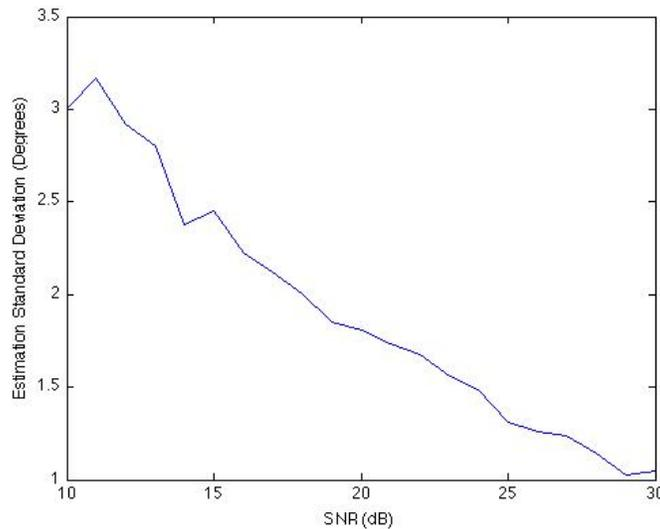
Fig. 2 – Standard deviation of angle estimation versus signal to noise ratio with a 9 element array.
