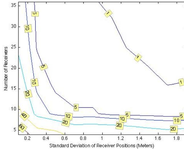
Fig. 3 – Contour plot showing the standard deviation of the angle estimation, in degrees, versus number of receivers and standard deviation of the randomly placed receivers.
