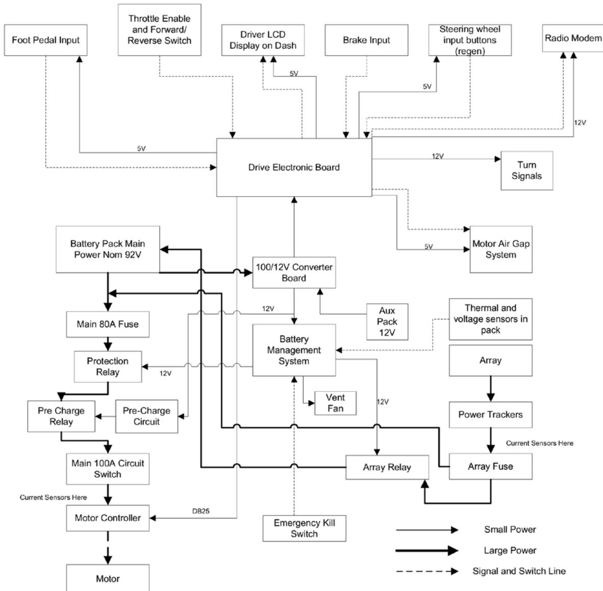
Figure 3. Solar Miner VII Electrical Subsystems
