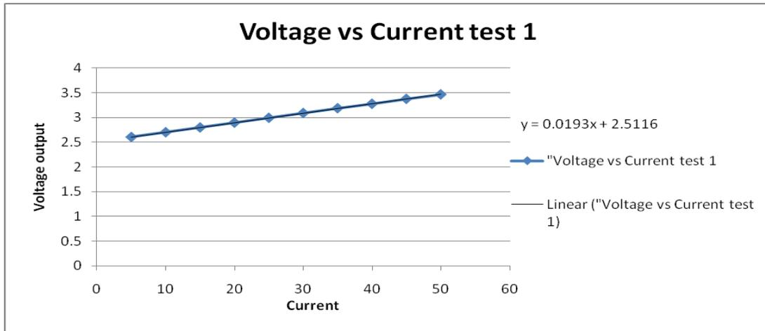
Figure 4. Calibration Data for Current Sensor – Test 1
