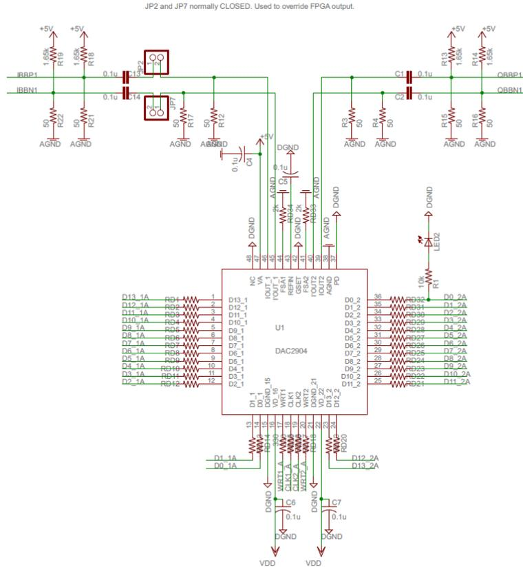
Figure A2. Digital to Analog Converter Schematic
