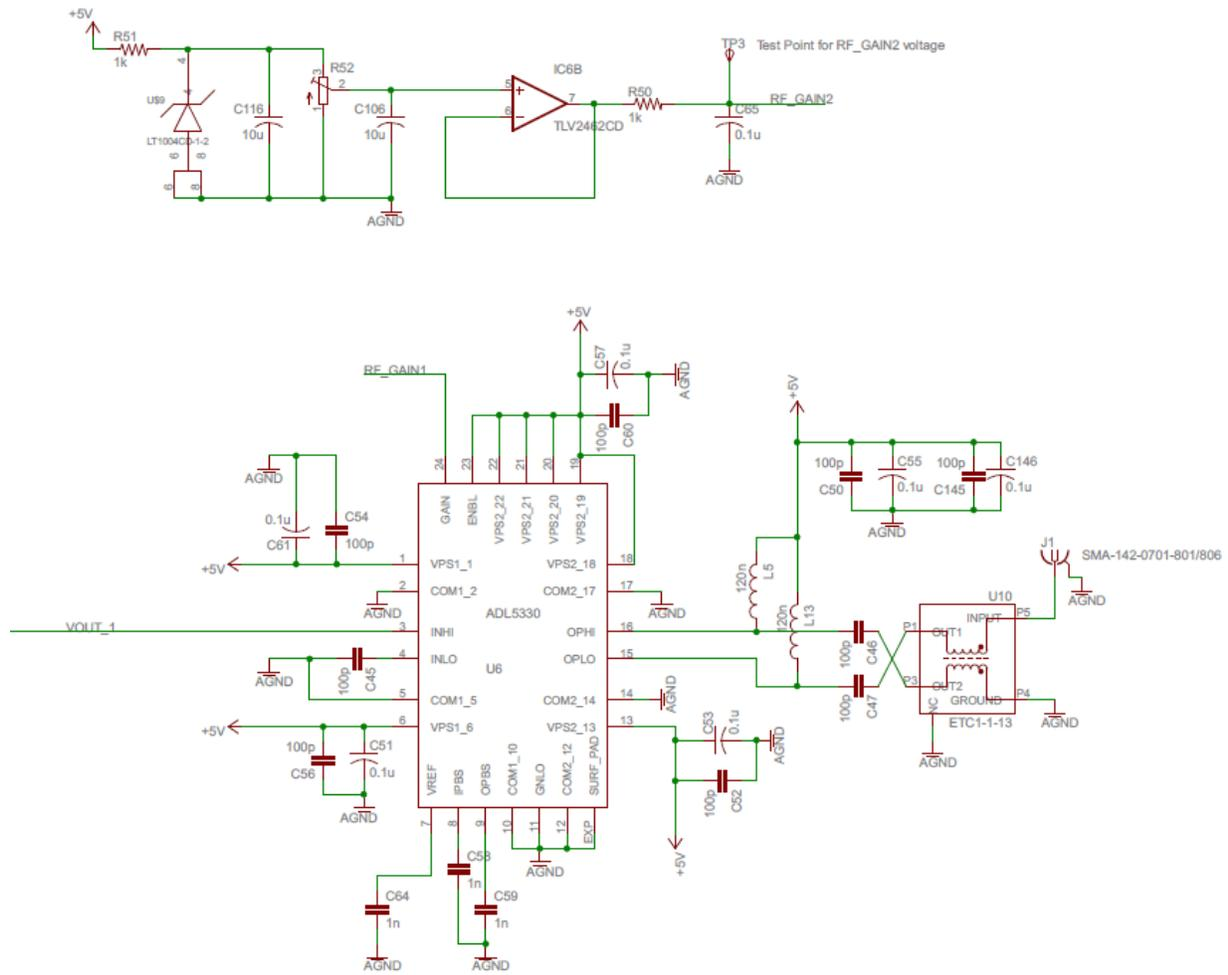
Figure A6. RF Amplifier Schematics
