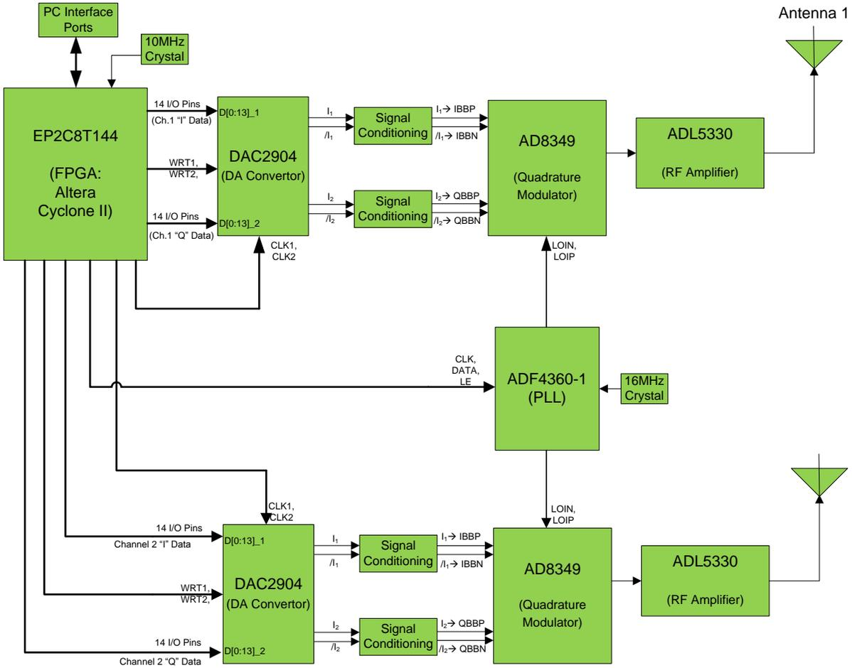
Figure 2. Detailed DART Block Diagram
