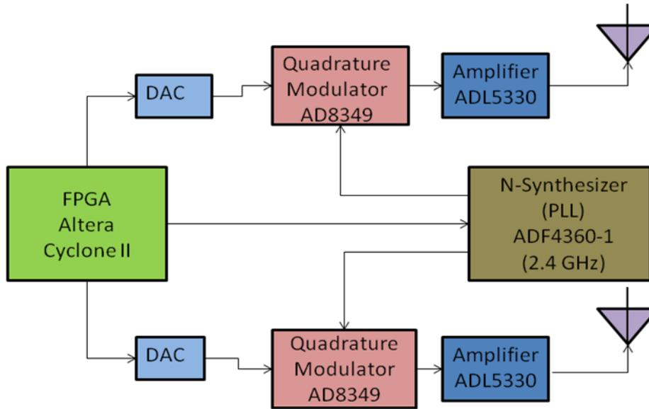
Figure 1. High Level Block Diagram of DART Board
