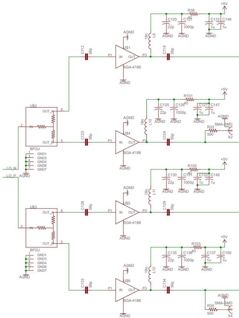
Figure A4. Power Splitter Schematic
