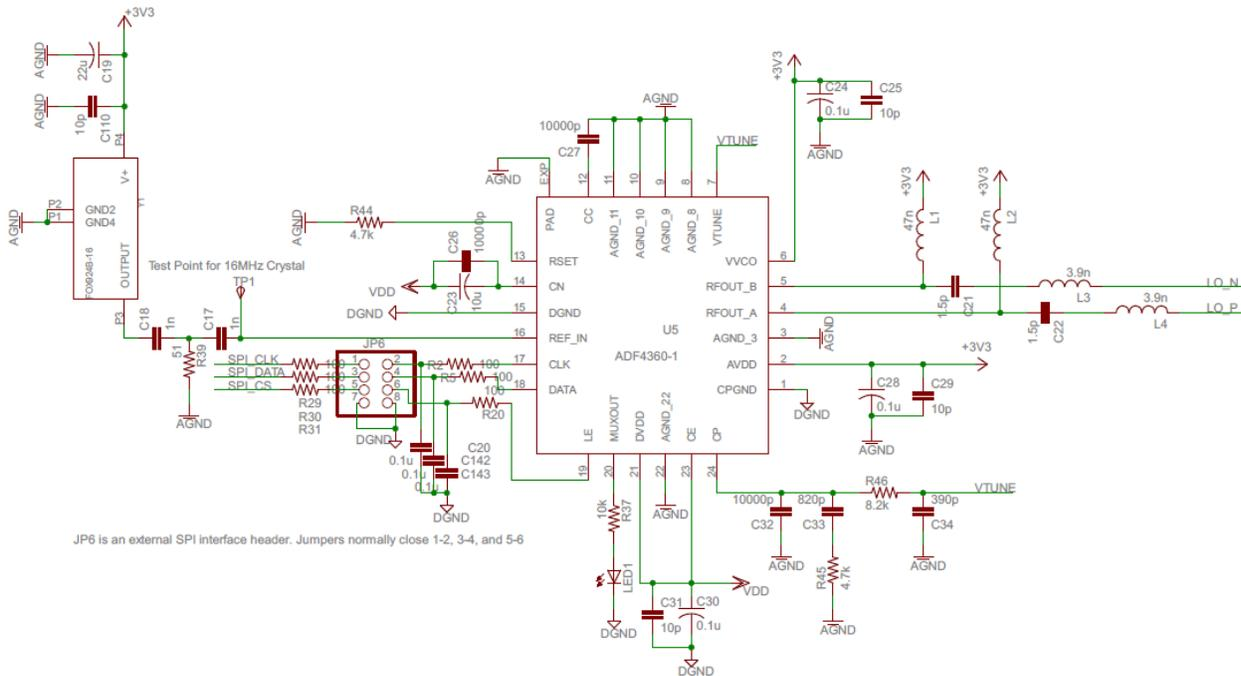
Figure A3. PLL Schematic
