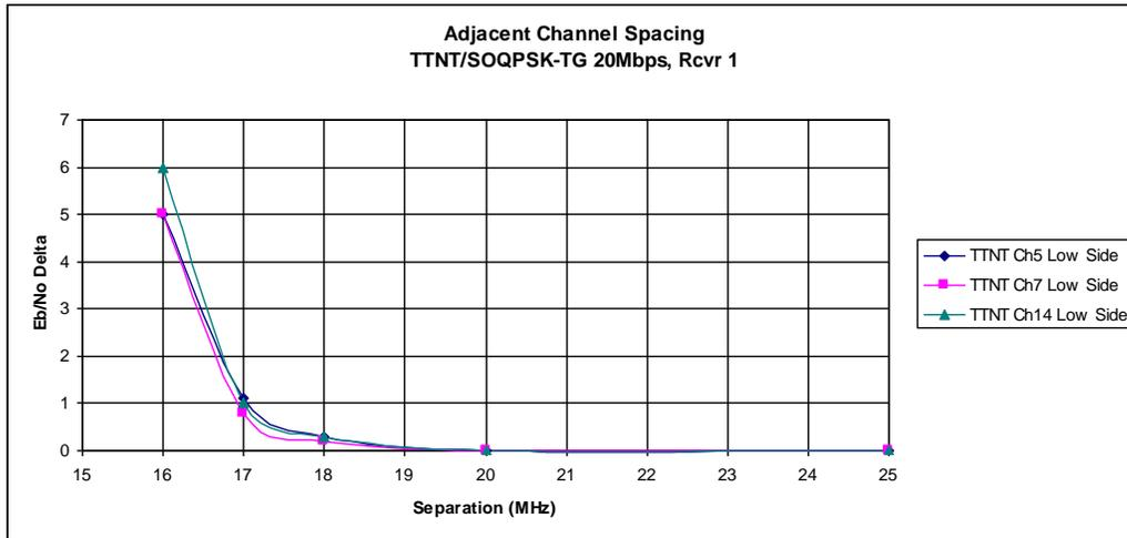
Figure 7 – Signal Separation vs. Delta Eb/No, 20Mbps SOQPSK-TG
