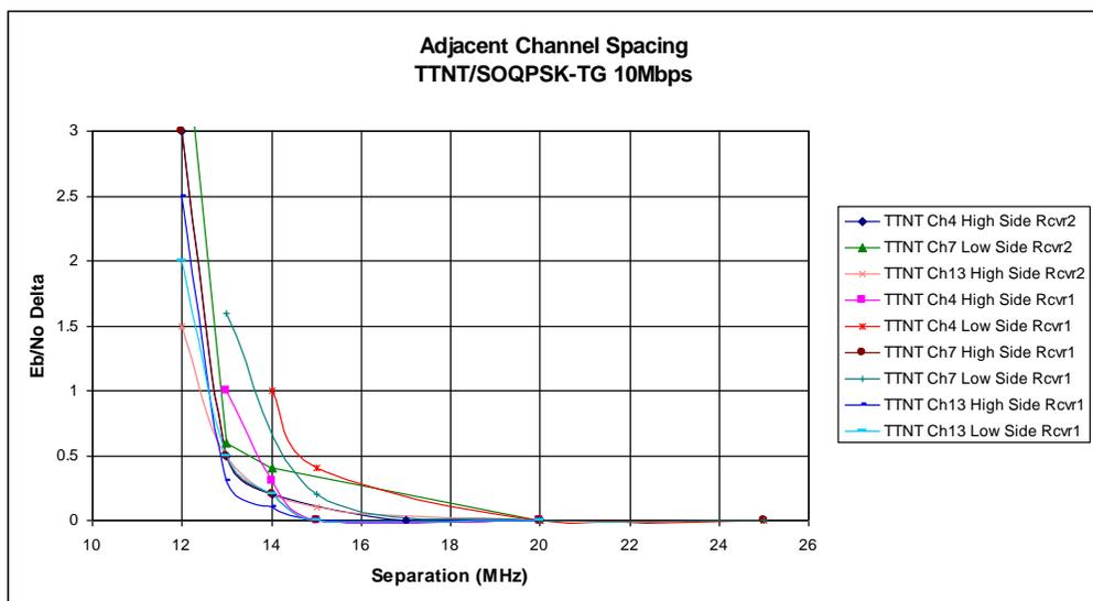
Figure 6 – Signal Separation vs. Delta Eb/No, 10Mbps SOQPSK-TG
