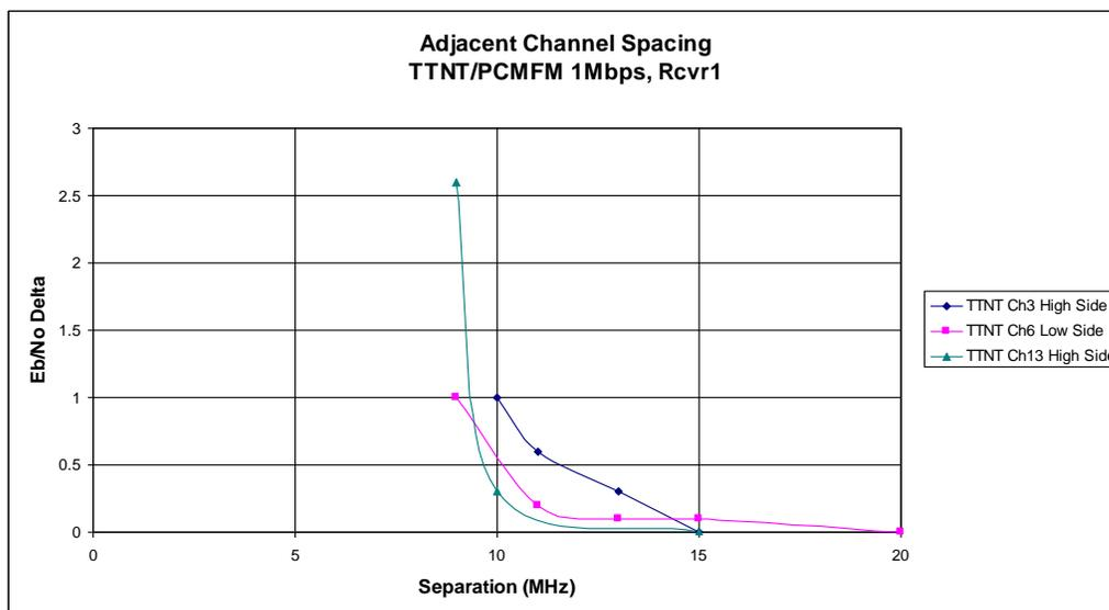
Figure 8 – Signal Separation vs. Delta Eb/No, 1Mbps PCM/FM
