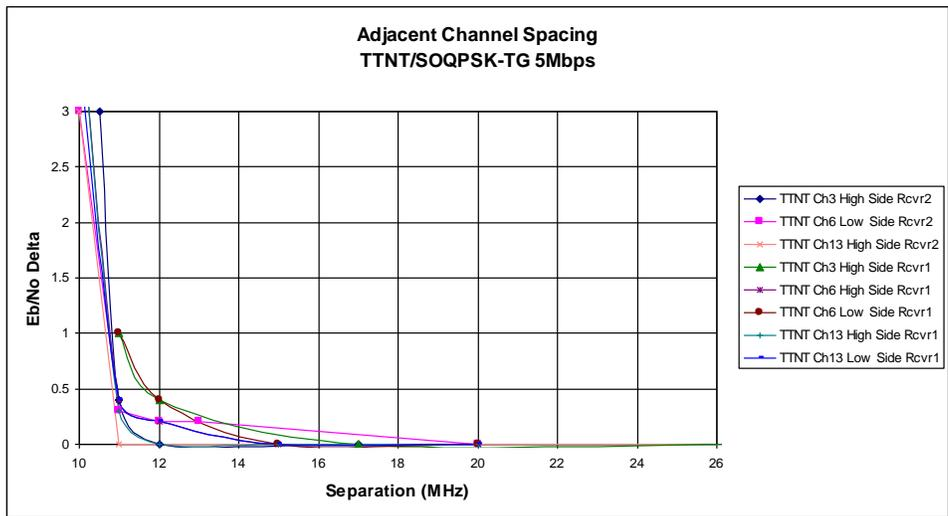
Figure 5 – Separation vs. Delta Eb/No, 5Mbps SOQPSK-TG
