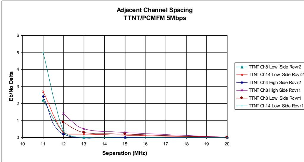
Figure 9 – Signal Separation vs. Delta Eb/No, 5Mbps PCM/FM
