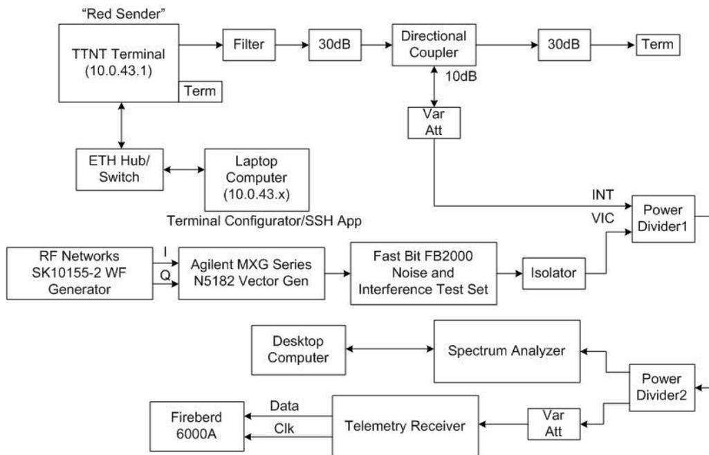
Figure 3 – ACI Testing Block Diagram
