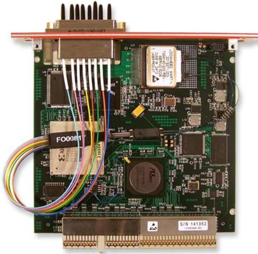
**Figure 4: JSF Fibre Channel Card for ASM**
