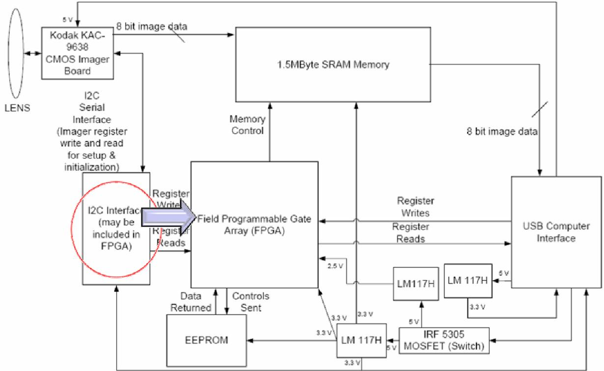
**Figure 6. Circuit Layout of the Previous Iteration RISA imager. The I<sup>2</sup>C controller circled in red is to be integrated into the FPGA as synthesized VHDL.**
