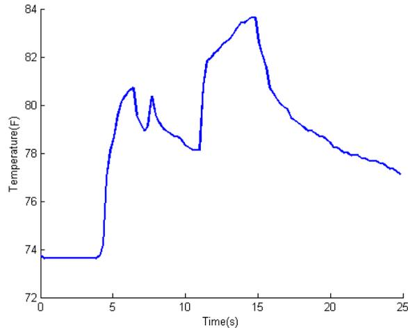
**Figure 7. Real-Time Temperature Plot using the Simple\_I<sup>2</sup>C IP Core for Communication with the TMP100 Temperature Sensor**
