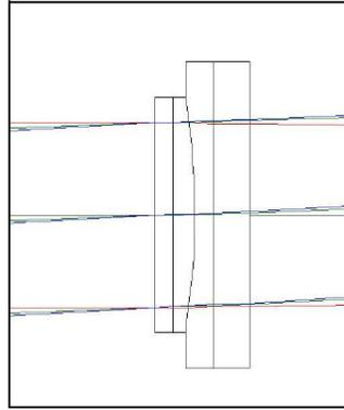
**Figure 1. 3D Liquid Lens Model**
