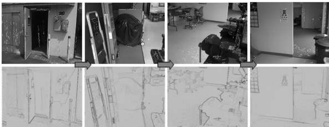
Figure 1: Image-based navigation using feature tracking; the user started moving from an outdoor to an indoor environment; in the figures several features of interest are extracted and tracked from one image to the next, facilitated the position fix.
