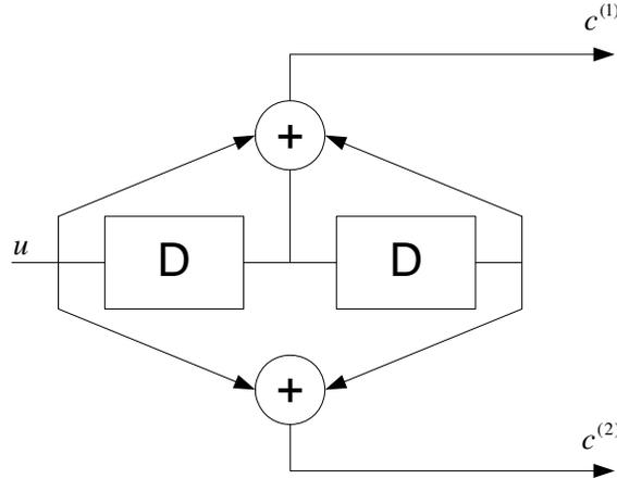
Figure 2: Block diagram of the rate-1/2 systematic convolutional encoder.
