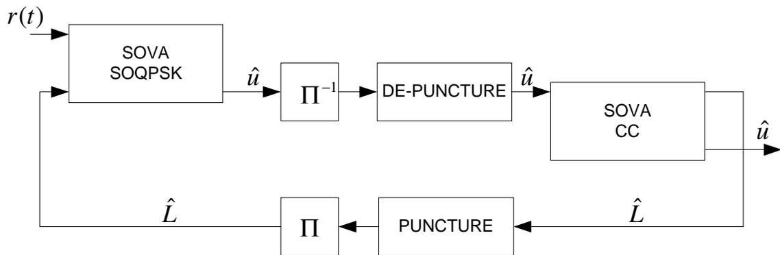
Figure 3: Block diagram of the decoder model for SOQPSK.
