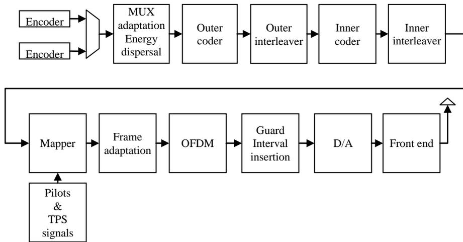
Figure 2. Functional block diagram of DVB-T system in non-hierarchical mode [4]
