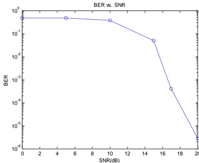
Figure 5. BER performance of designed DVB-T system under multipath channel
