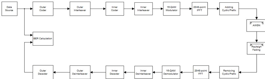
Figure 4. Designed DVB-T baseband system in Simulink
