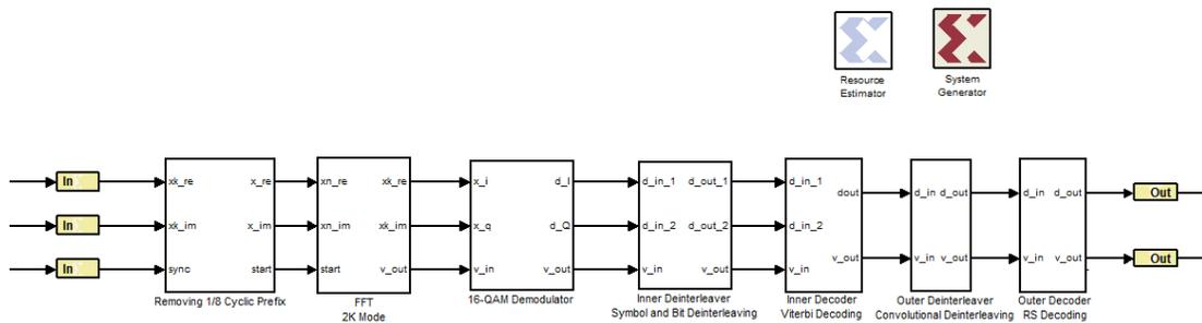
Figure 7. DVB-T baseband receiver constructed by System Generator
