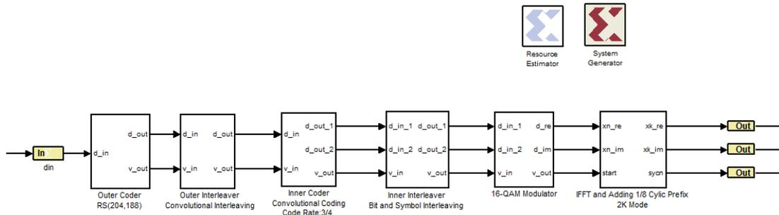
Figure 6. DVB-T baseband transmitter constructed by System Generator
