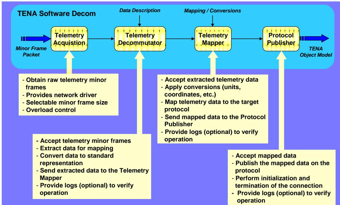
Figure 5. TSDS Architecture
