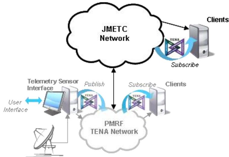
**Figure 1. JMETC Network Node Conceptual Diagram**
