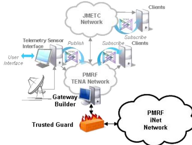
**Figure 2. iNet Connectivity Conceptual Diagram**
