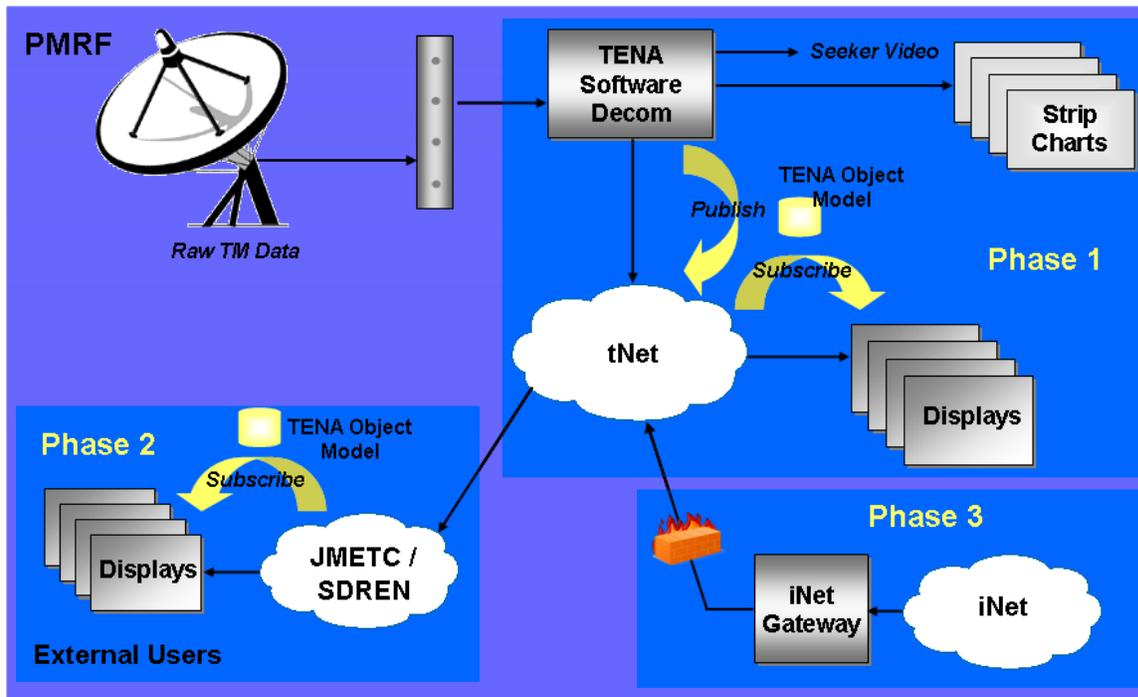
**Figure 4. TSDS implementation within PMRF and JMETC network infrastructure**
