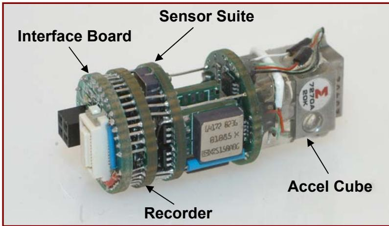
Figure 4: Electronics Stack
