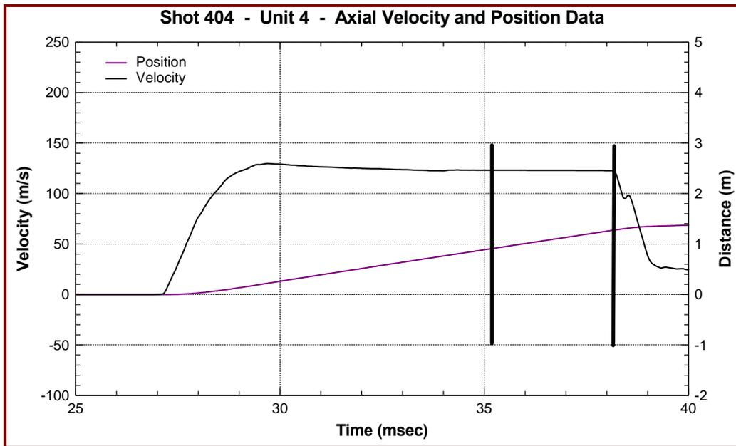
Figure 26: Axial Velocity and Position Data from Unit #4 Shot #1
