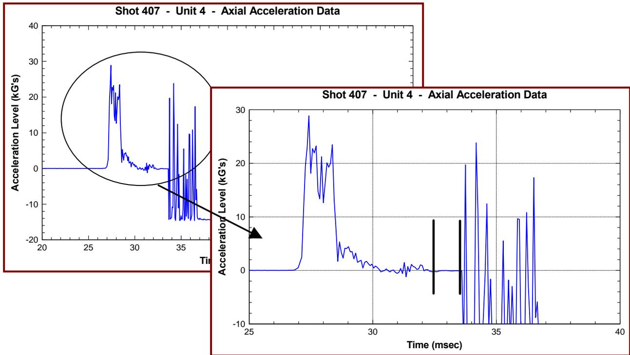
Figures 27 and 28: Axial Acceleration Data from Unit #4 Shot #2
