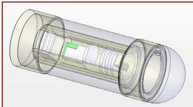
Figure 7: Electronics Module Inserted into Projectile
