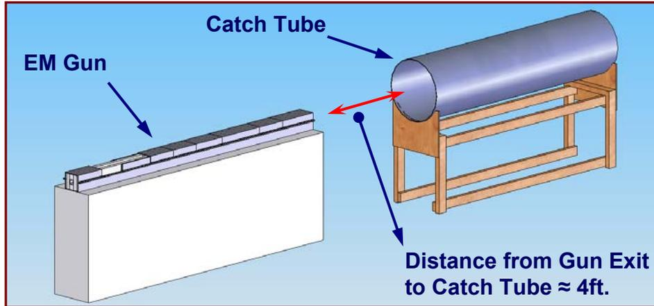
Figure 8: Experimental Test Setup
