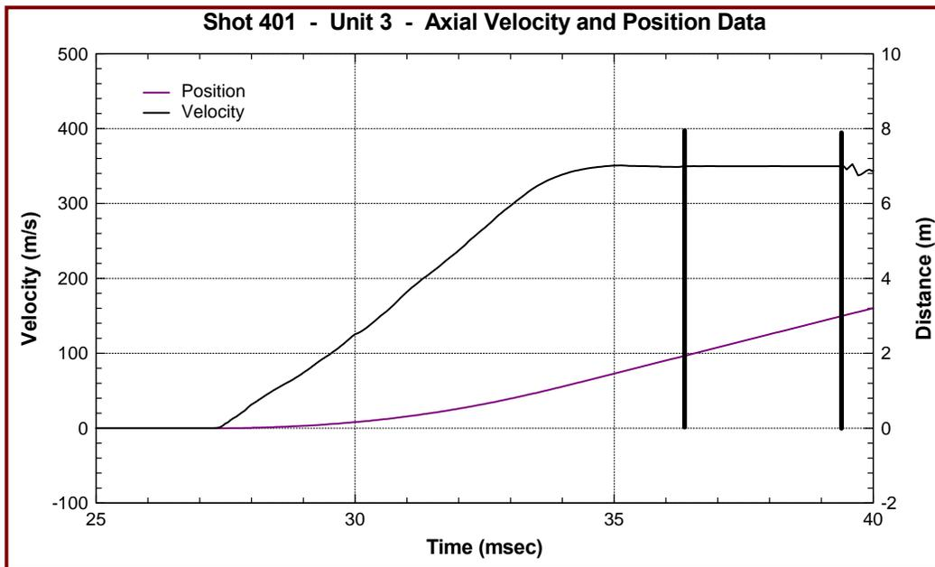
Figure 21: Axial Velocity and Position Data from Unit #3 Shot #1
