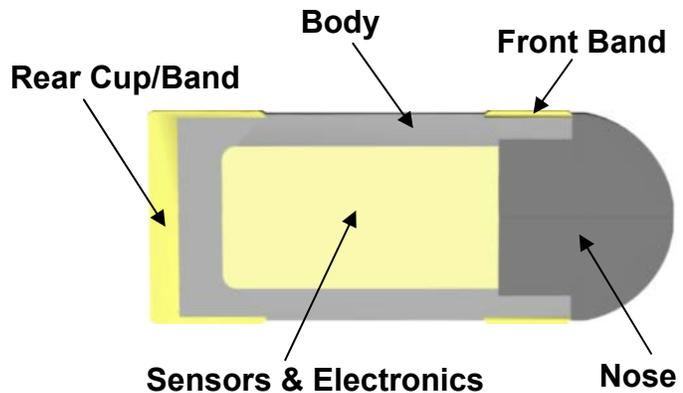
Figure 2: Cross-section of Projectile
