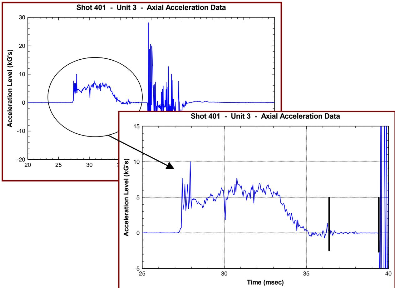
Figures 19 and 20: Axial Acceleration Data from Unit #3 Shot #1
