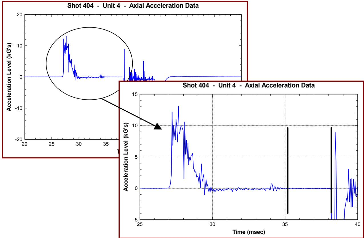
Figures 24 and 25: Axial Acceleration Data from Unit #4 Shot #1
