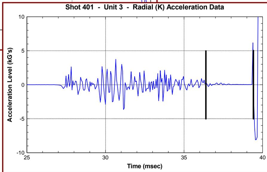
Figures 22 and 23: Radial Acceleration Data from Unit #3 Shot #1
