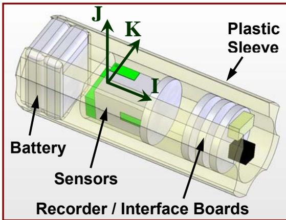
Figure 5: Electronics Module Concept
