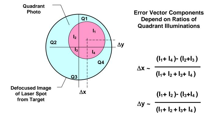
Figure 2. Schematic diagram of optical quad-detector with the standard relations for measured photo current and laser spot offset in x and y directions required for determining the position of the reflected laser energy from target designator.
