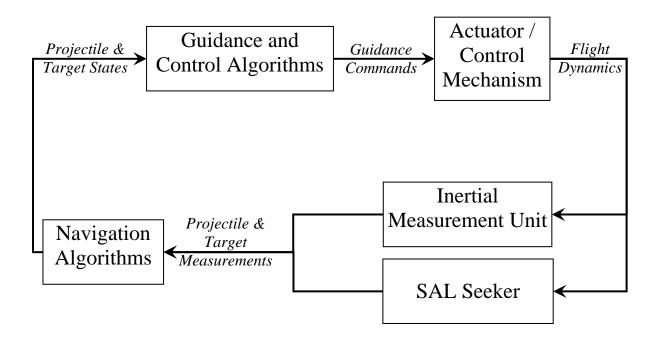
Figure 5. Block Diagram of SAL Seeker Implementation in GNC System
