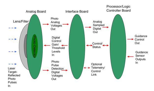
Figure 4. SAL seeker electronic board level block diagram.
