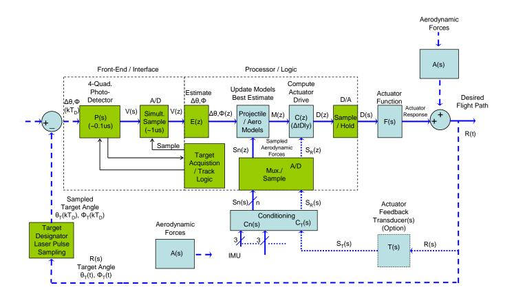
Figure 3. SAL seeker system control diagram.
