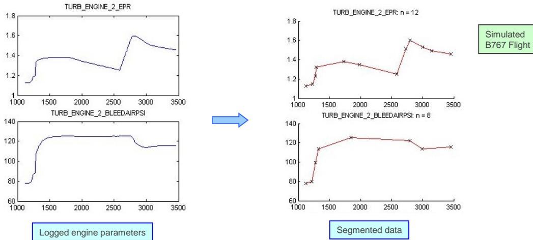
**Figure 2: Examples of raw flight data channels with their segmented versions**
