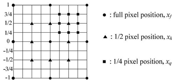
Fig. 4. Logarithm search method using interpolated image.
