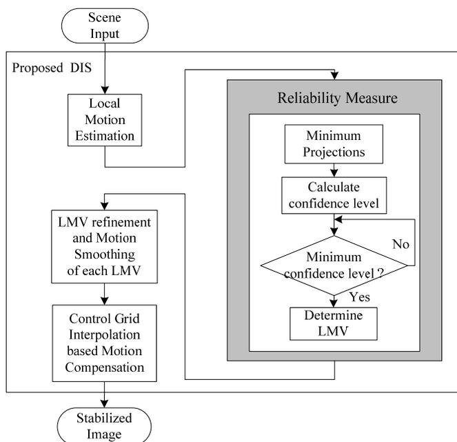
Fig. 1. Flowchart of the proposed DIS algorithm.
