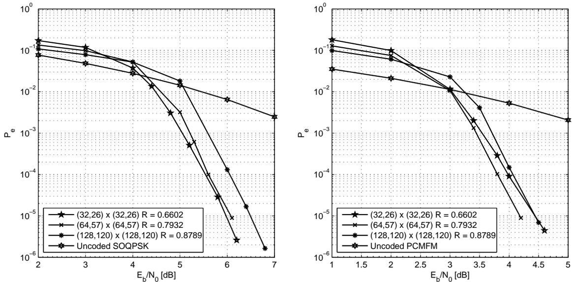
(a) Simulation Results for Coherent TPC-SOQPSK-TG. (b) Simulation Results for Coherent TPC-PCM/FM.
