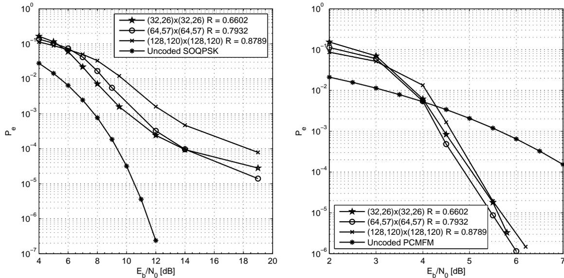
(a) Simulation Results for Non-Coherent TPC-SOQPSK-TG. (b) Simulation Results for Non-Coherent TPC-PCM/FM.
