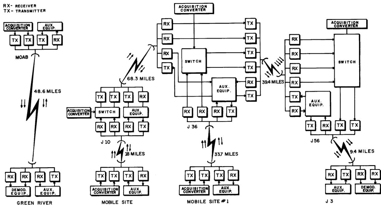
Fig. 6-Microwave Relay System
