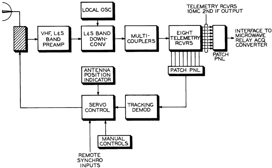
Fig. 5-Telemetry Acquisition System
