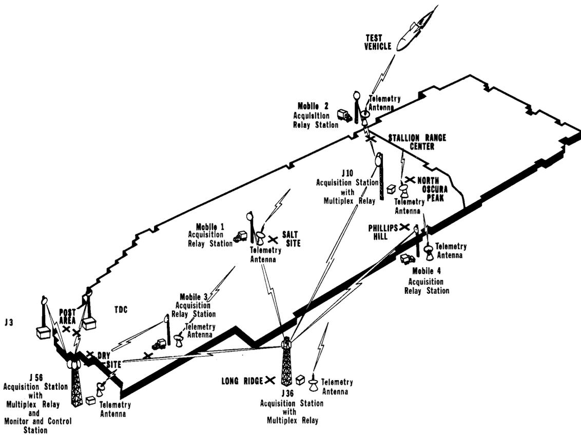
Fig. 4-Telemetry System
