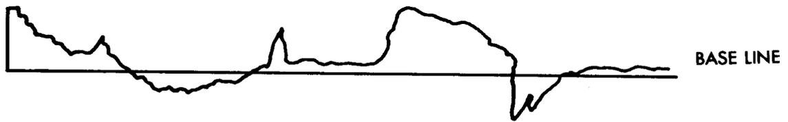
Fig. No. 3 Typical PPI Radar Presentation When the Recorder Exhibits Restricted Low Frequency Response
