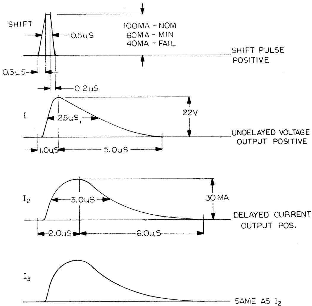
**Fig. 4 - Delay Logic Timing Diagram**
