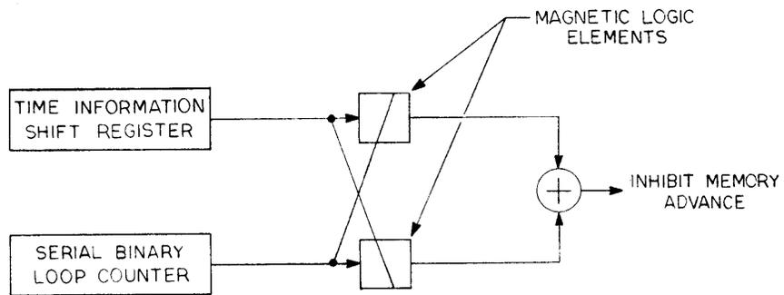
**Fig. 9 - Serial Time Comparison**
