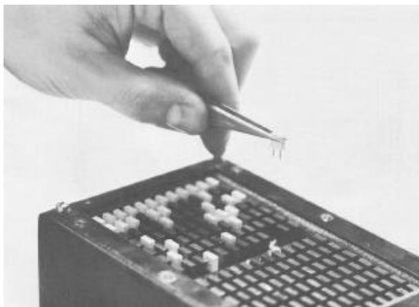
**Fig. 12 - Resistor Plug Matrix Programming**
