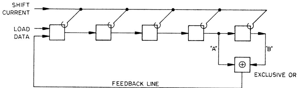
**Fig. 7 - Linear Feedback Register**
