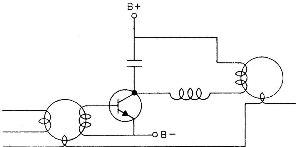
**Fig. 6 - Core Transistor Non-Regenerative Logic Schematic**
