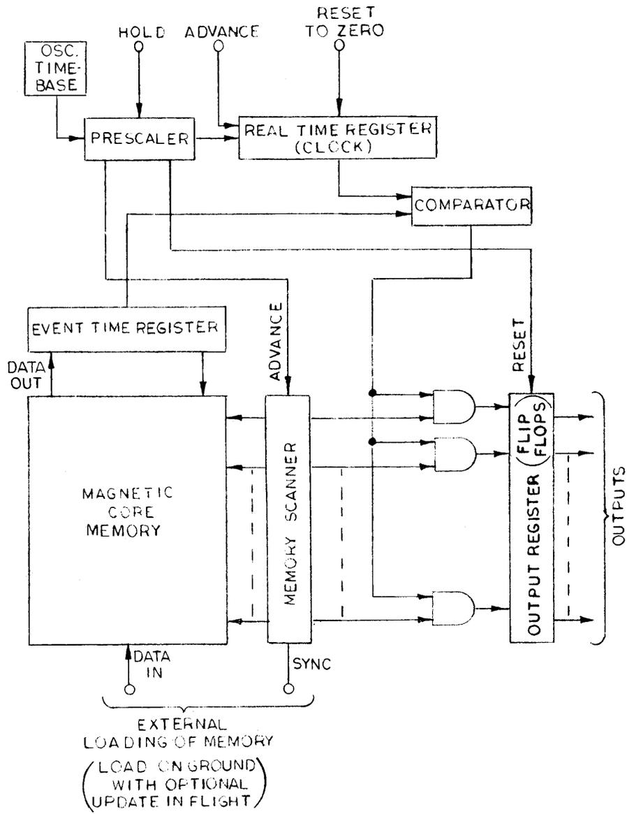
**Fig. 11 - Electronic Sequence Timer with Program Memory**
