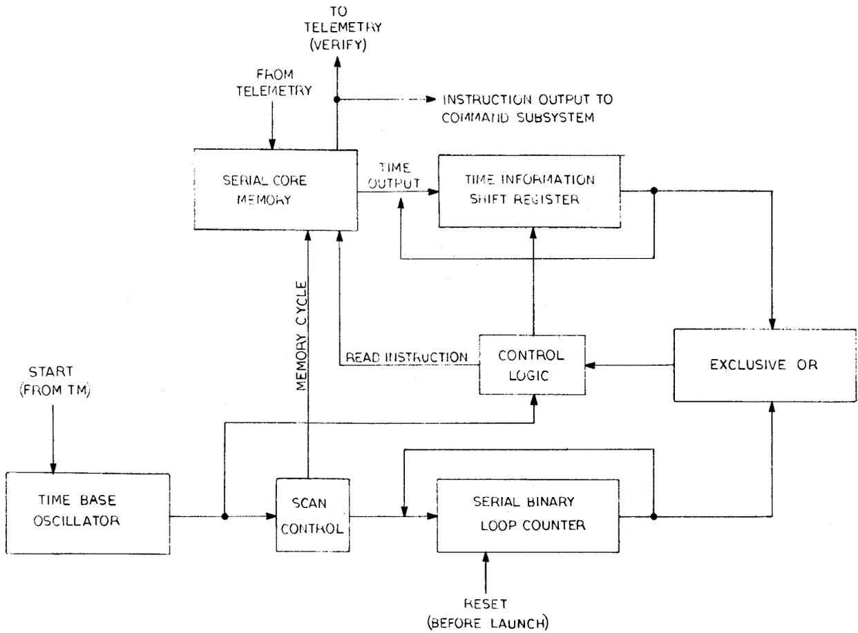
**Fig. 1 - Magnetic Sequential Programmer Block Diagram**
