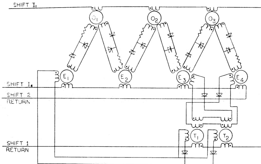
**Fig. 2 - Two Phase Core Diode Register**
