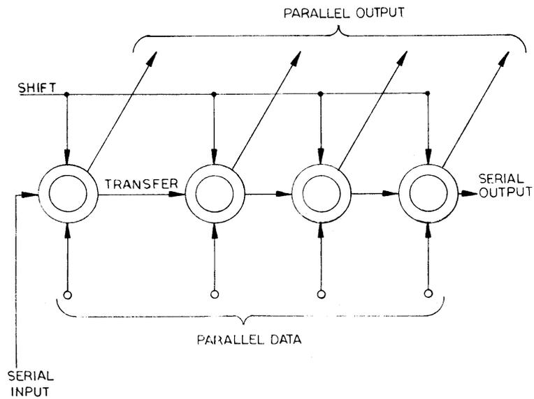
**Fig.10 - Core Presetting: Parallel to Serial Conversion in a Shift Register**
