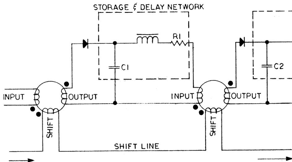
**Fig. 3 - Core-Diode with Delay**
