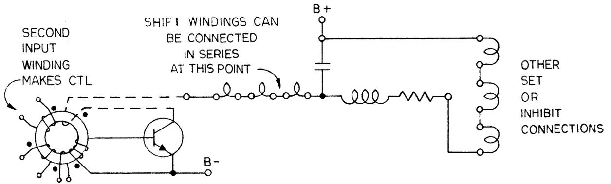
**Fig. 5 - Regenerative Core Logic Schematic**
