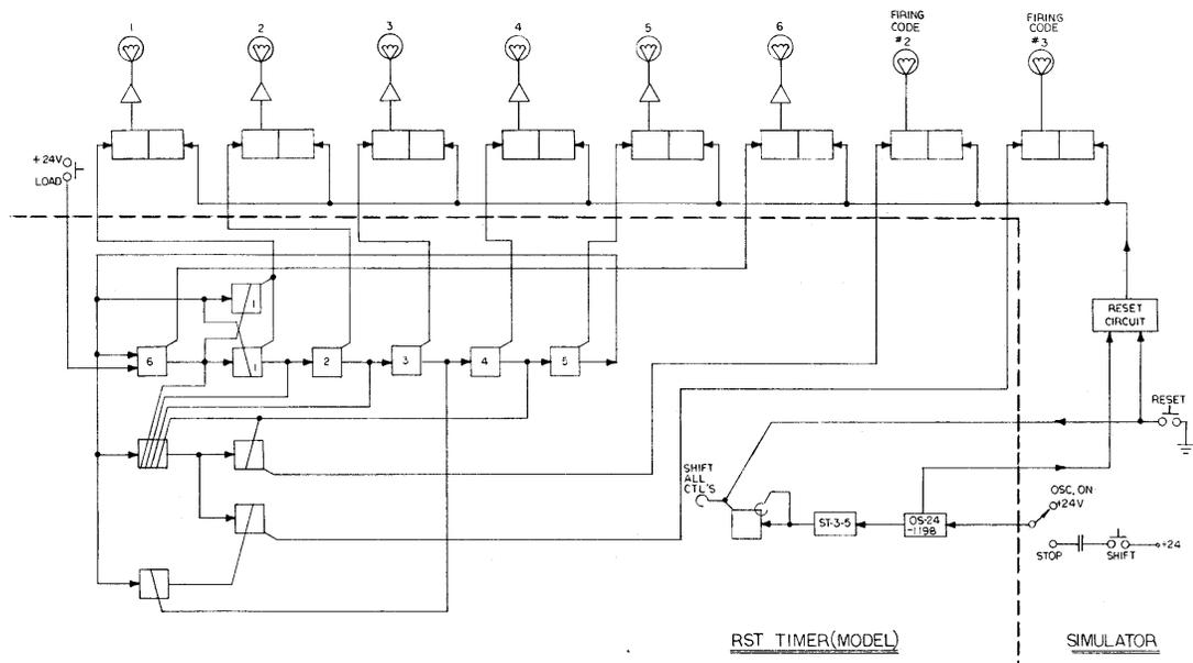
**Fig. 8 - Linear Feedback Timer with Decoder**
