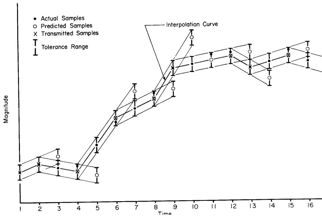
**Fig. A-6 - First Order, Fixed Corridor, Adjusted Preceding Sample Transmitted (FFA).**
