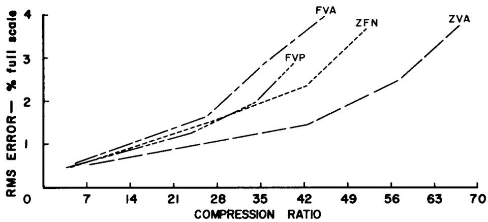
**Fig. 5 - Evaluation of Algorithms During Entire Flight of SA-10 Using Pressure Measurement Data.**
