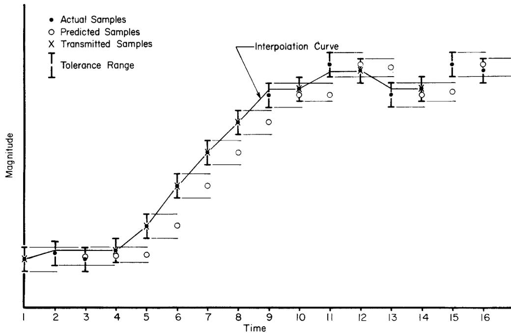
**Fig. A-2 - Zero Order, Variable Corridor, Preceding Sample Transmitted (ZVP).**
