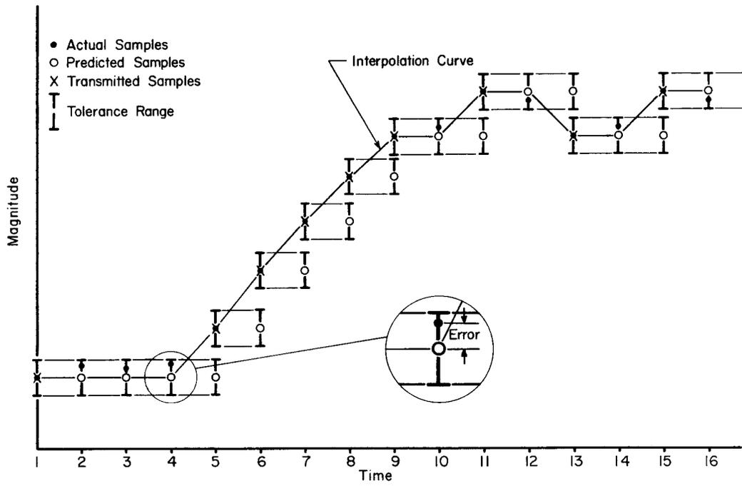
**Fig. A-1 - Zero Order, Fixed Corridor, Non-redundant Sample Transmitted (ZFN).**
