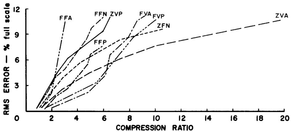
Fig. 4 - Evaluation of Algorithms Using Synthesized Data.
