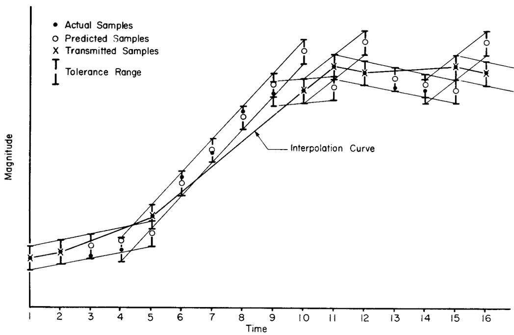
**Fig. A-4 - First Order, Fixed Corridor, Non-redundant Sample Transmitted (FFN).**
