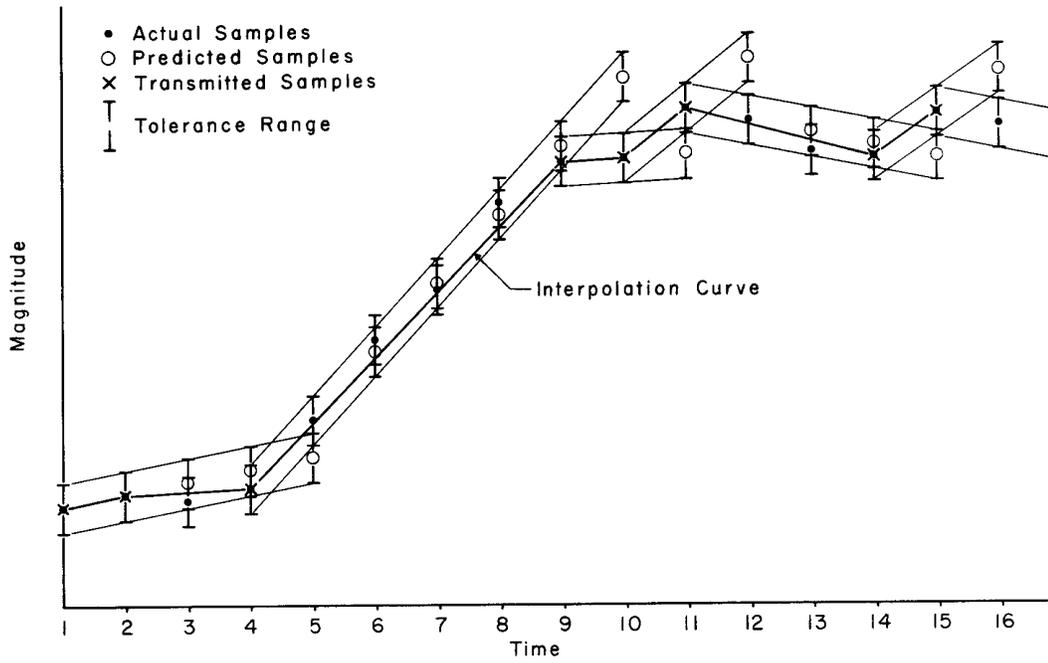
**Fig. A-5 - First Order, Fixed Corridor, Preceding Sample Transmitted (FFP).**
