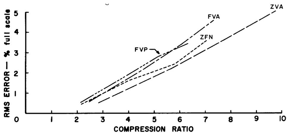
**Fig. 6 - Evaluation of Algorithms During Ignition of SA-10 Using Pressure Measurement Data.**
