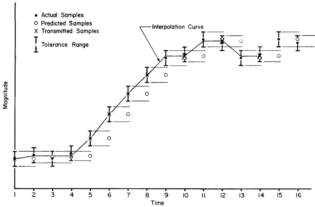
**Fig. A-3 - Zero Order, Variable Corridor, Adjusted Preceding Sample Transmitted (ZVA).**
