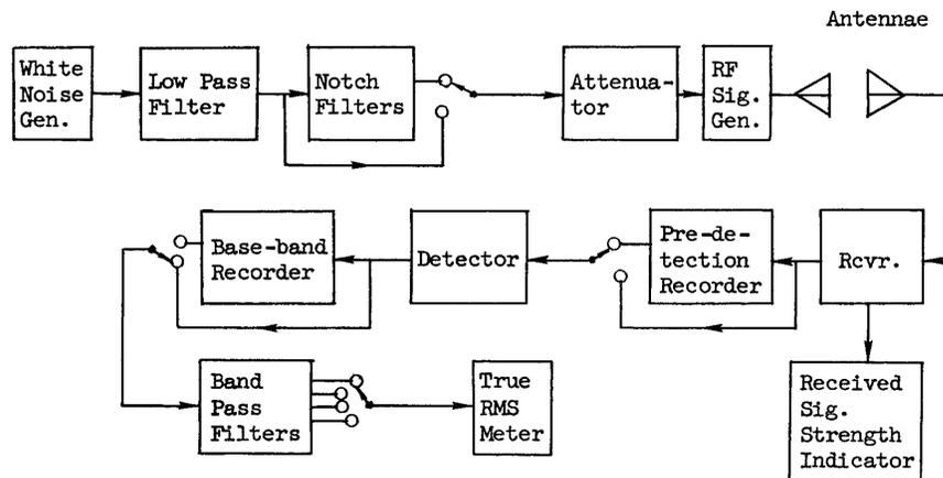
Figure 1. Notch Noise Tester
