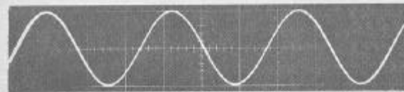
FIGURE 8. FM/FM CHANNEL C RESPONSE 1 Kc Sine Wave 1.2 Kc Filter
