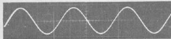
FIGURE 9. PAM/FM RESPONSE 3125 Sample/Sec 1 Kc Sine Wave 1.2 Kc Filter
