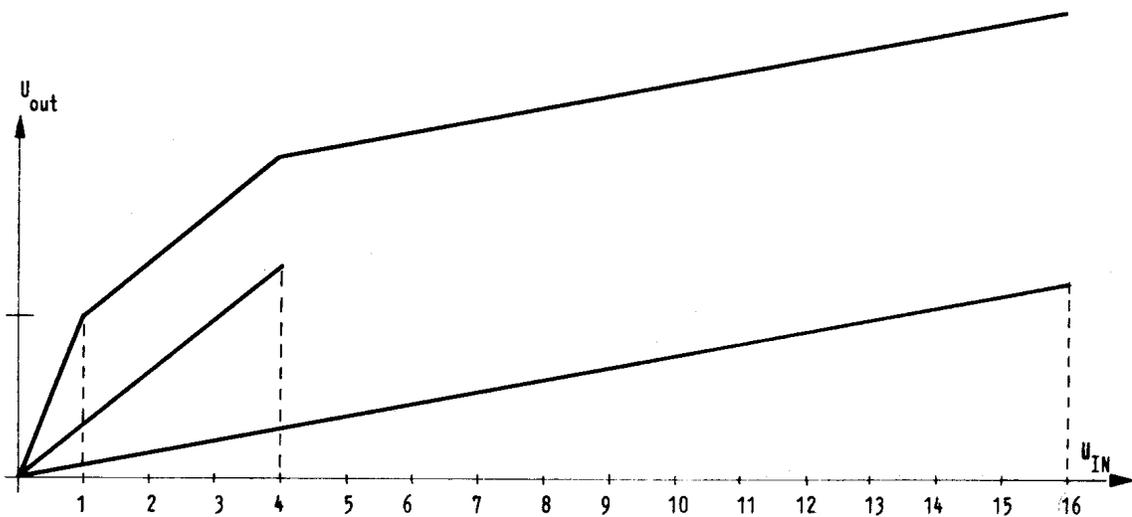
Figure 22 - Characteristics for a 2 Stage Saturating Amplifier with a Stage Amplification of 4 and Corresponding Straight - Line Approximation of the Logarithm
