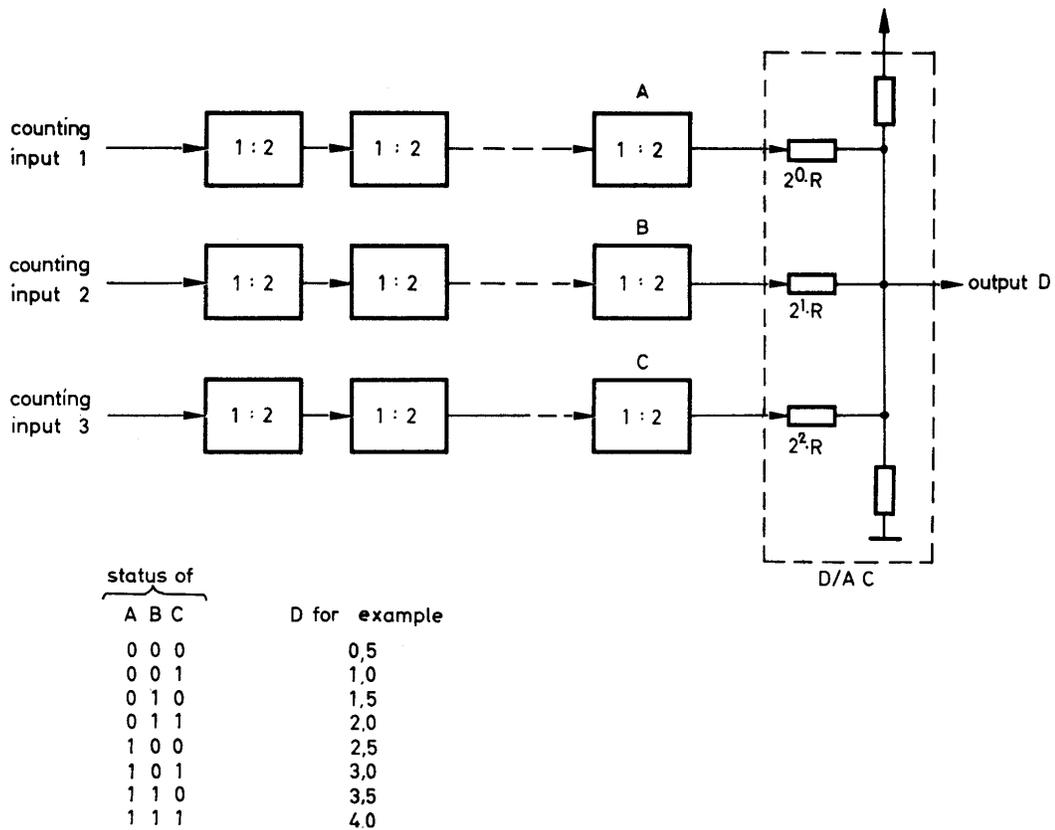
Figure 4 - Conversion from a binary to an 8 level system
