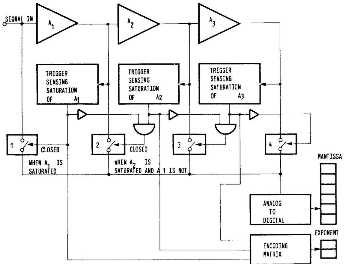
Figure 21 - The Saturating Amplifier Concept
