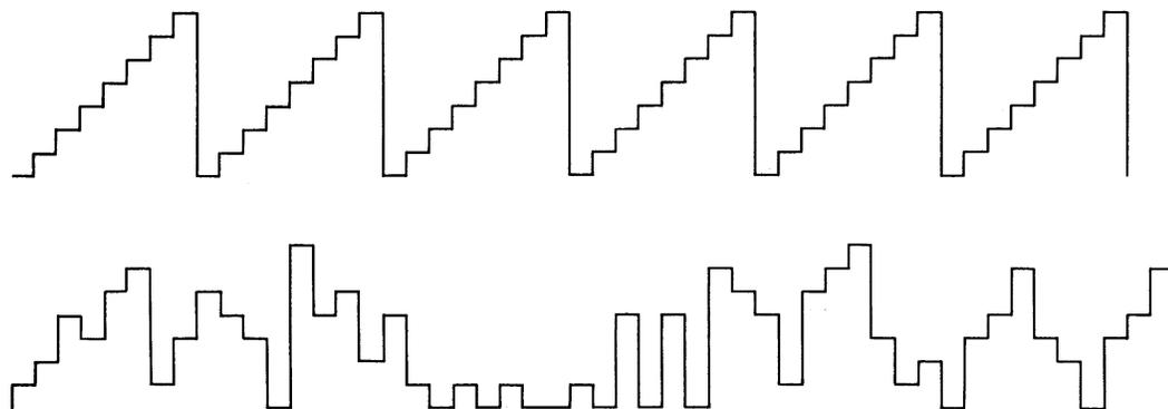
Figure 6 - Typical 8 - Level - Waveforms
