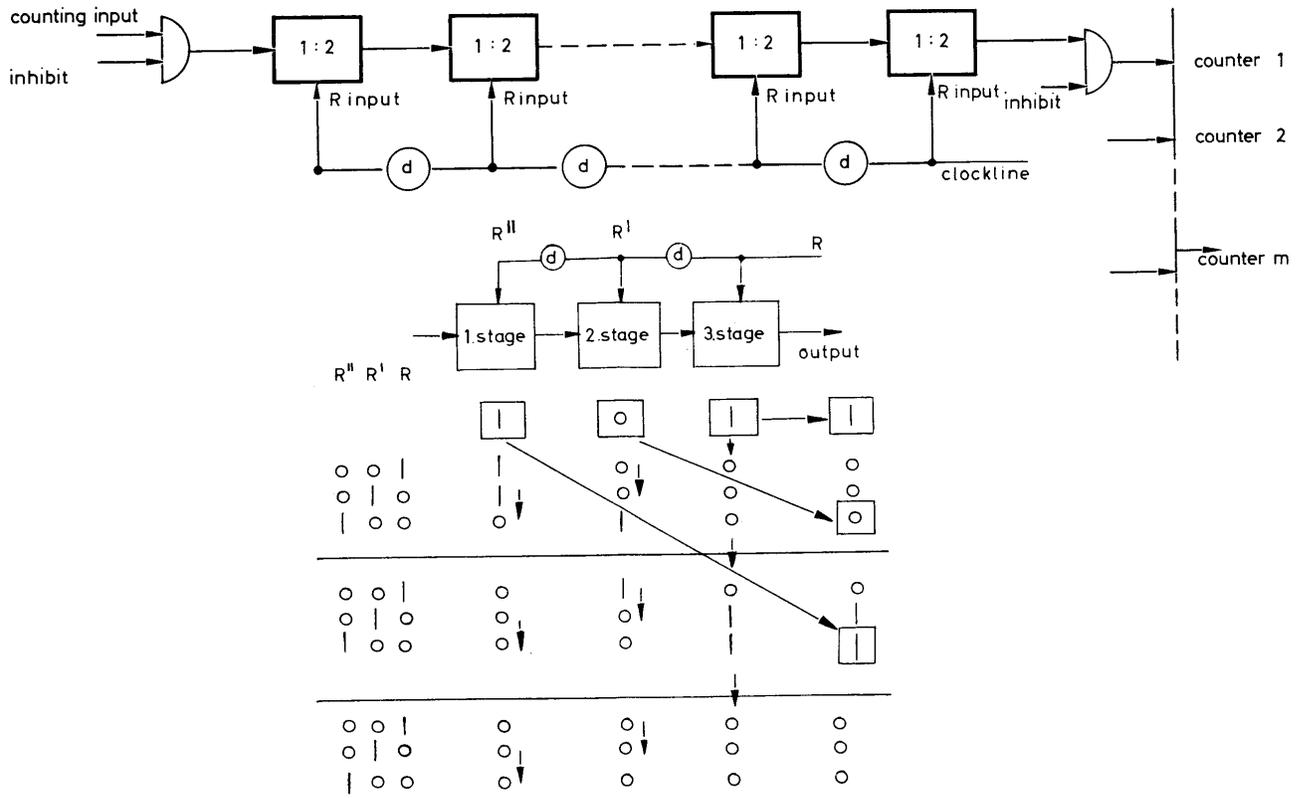
**Figure 11 - Binary Counter with Delay Units**
