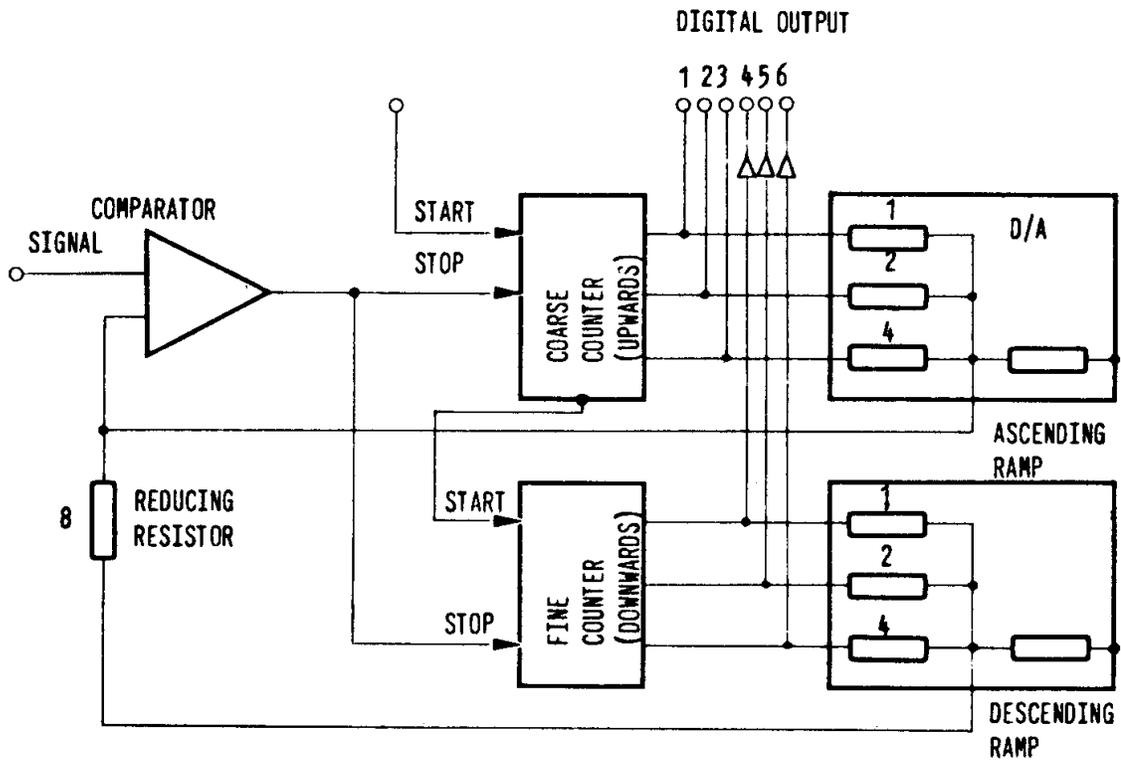
Figure 24 - Block Diagram of the Encoder
