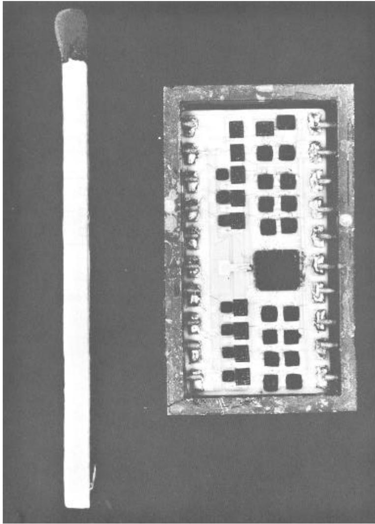
**Figure 25 - One of the 5 Thick-Film Flatpacks Comprising a 14 Bit ADC**
