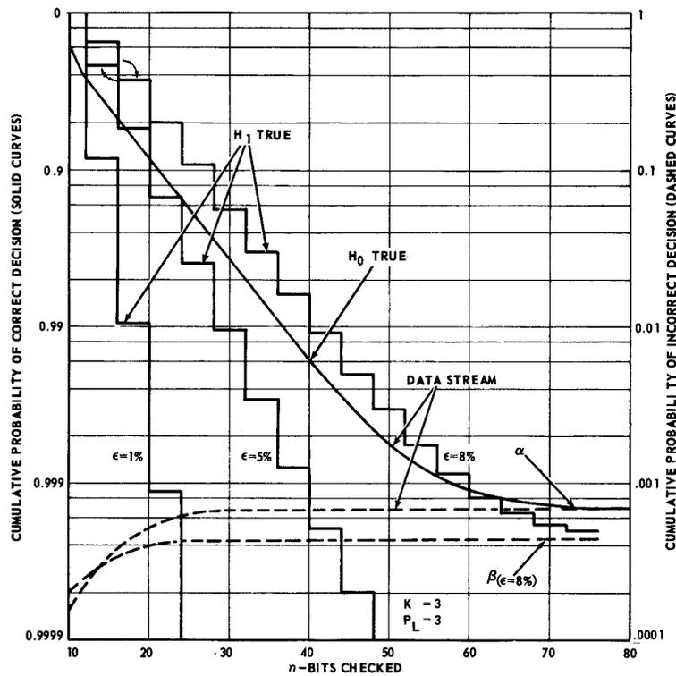
Fig. 7 - SPRT Decision Speed for Different Error Rates and  $K=3$
