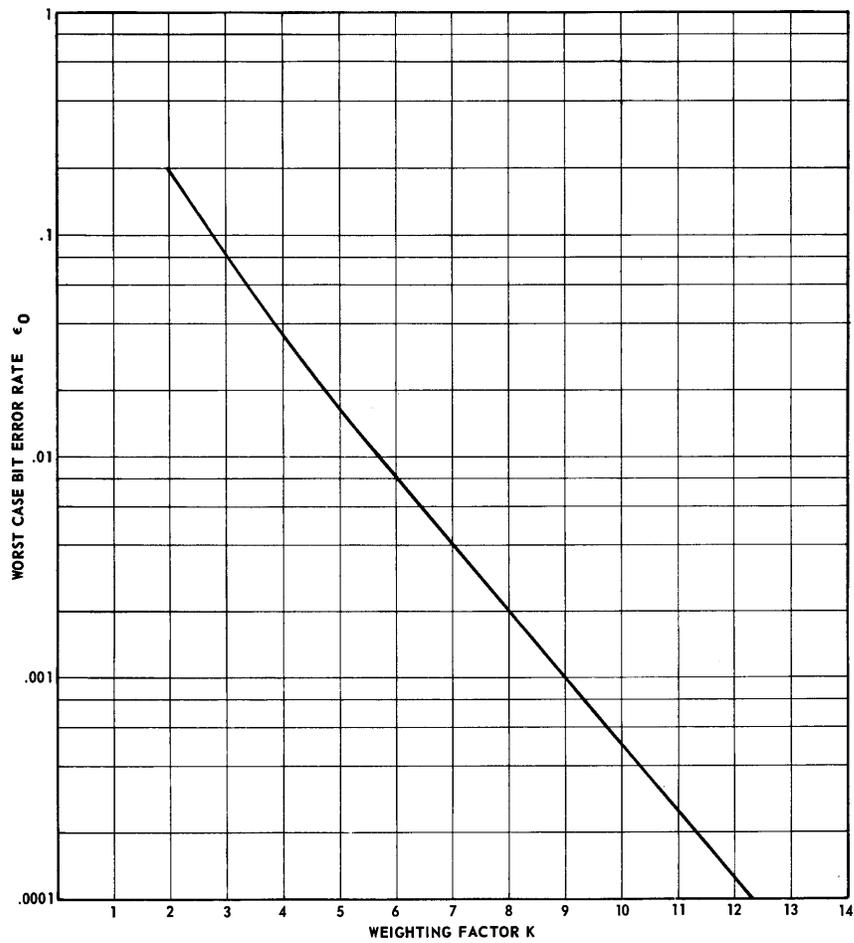
**Fig. 2 - Weighting Factor K as Function of Worst Case Bit Error Rate**
