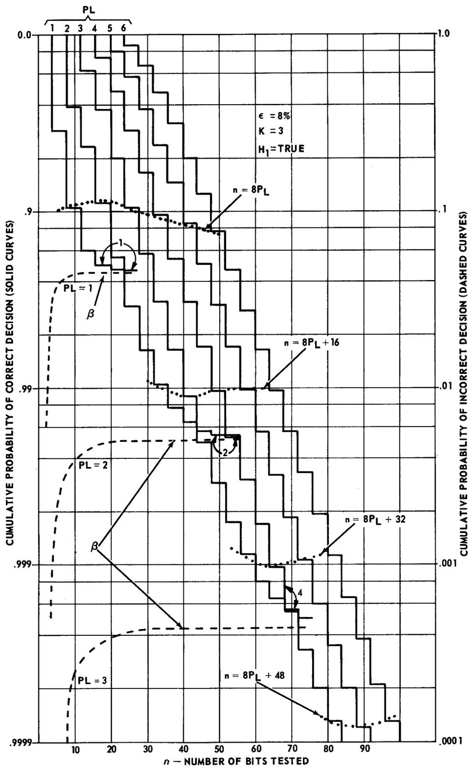
Fig. 8 - SPRT Decision Speed for Different Programmed Limits  $P_L$
