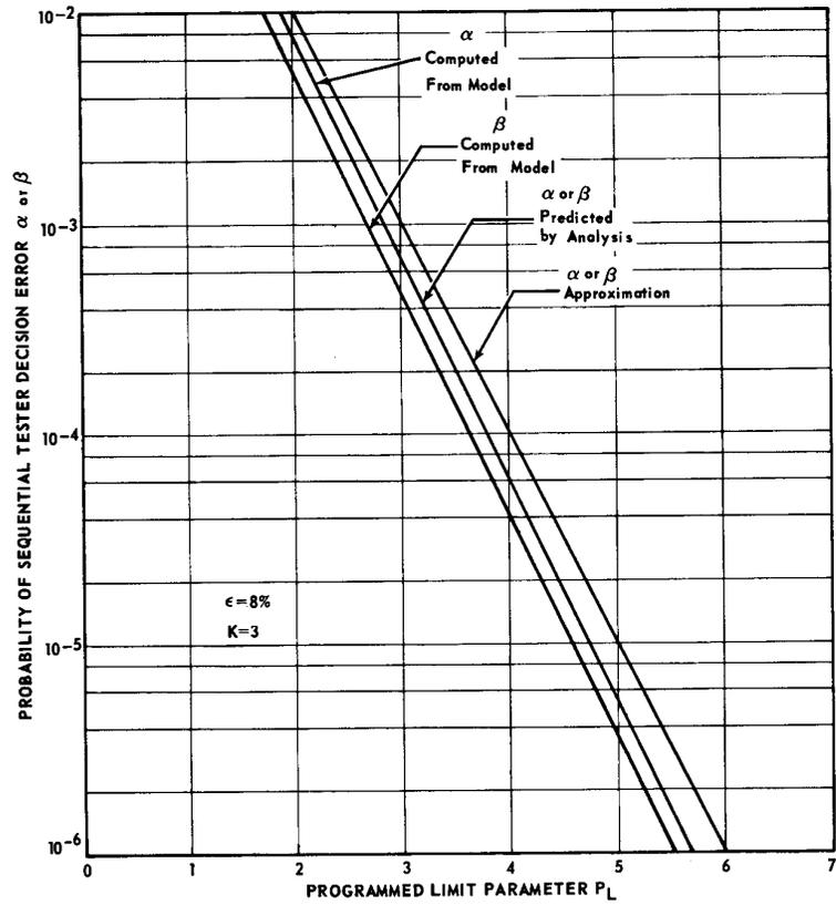
Fig. 6 -  $\alpha$  and  $\beta$  as Function of Programmed Limit Parameter  $P_L$
