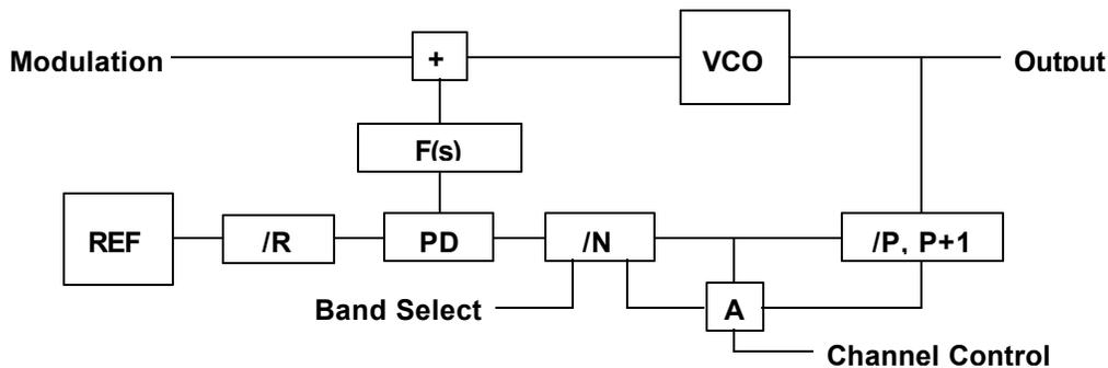
Figure 2. Topology for Phase Locked Loop Circuit.
