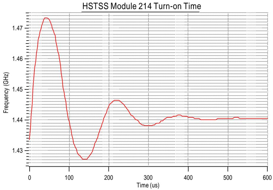
Figure 5. Turn-on time for Phase Locked L-Band Transmitter
