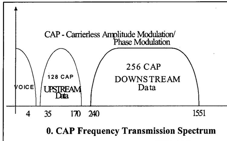
Figure 0 illustrates CAP frequency spectrum. It can be seen that voice channel occupies the smallest part of the spectrum (0.4.3KHz) and can be separated (filtered) from the data frequency spectrum.
