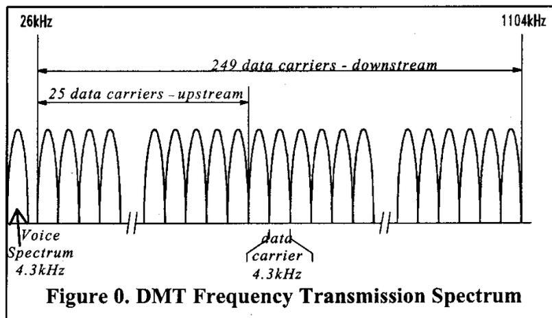
**DMT** (*see below*) is a version of multi-carrier modulation in which incoming data is collected and then distributed over a number of small individual carriers, each of which uses a form of QAM modulation. DMT is the basis of ANSI Standard T1.413 and is becoming the prevailing standard, considered to be more resilient to electrical noise (*DMT is the preferred standard in Defence forces*).
