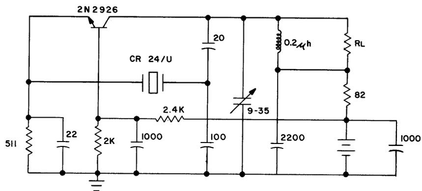
**Figure 3 - 50 MHz Crystal Oscillator.**
