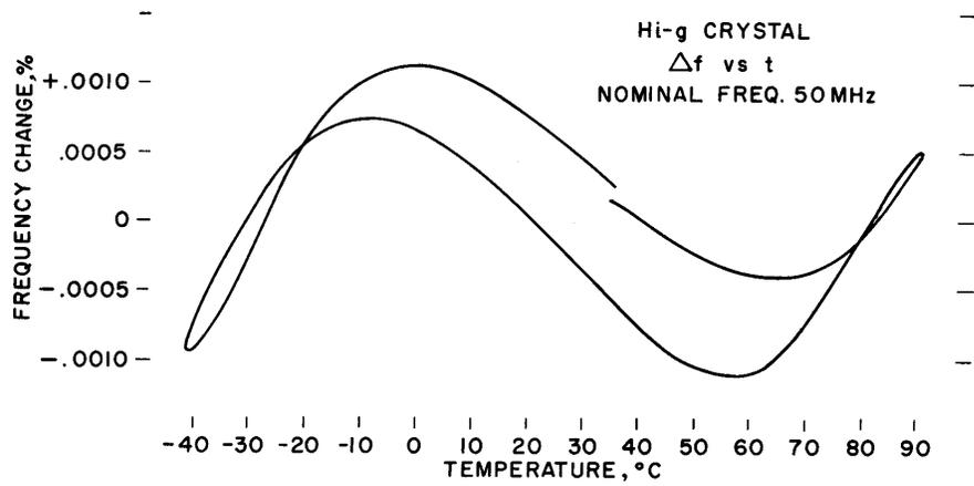
**Figure 6 - Hi-G Crystal Temperature Curve.**
