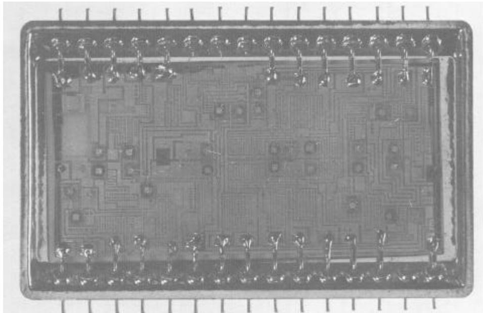
**Figure 5. Differential Amplifier Photograph**
