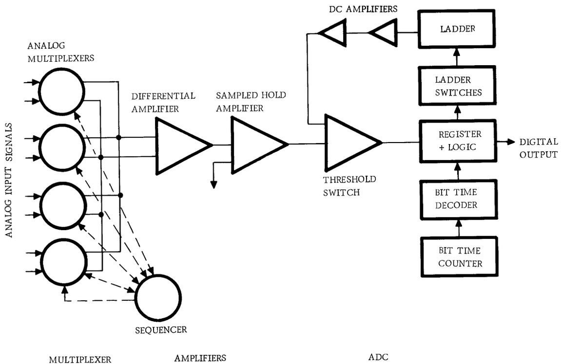
**Figure 1. PCM Telemetry System Block Diagram**
