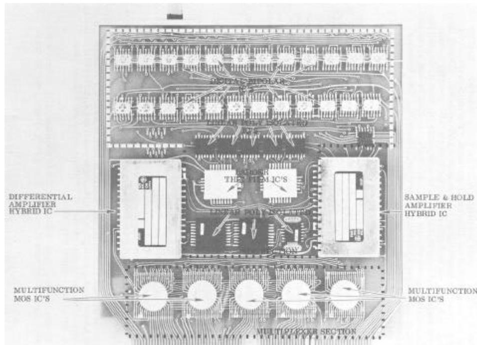
**Figure 2. PCM Telemetry Module**
