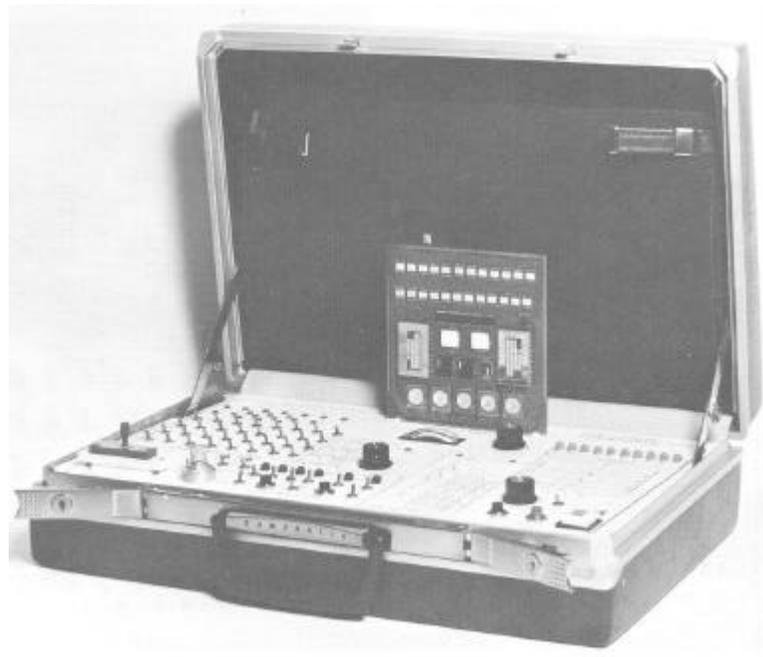
**Figure 6. PCM Telemetry Demonstrator**
