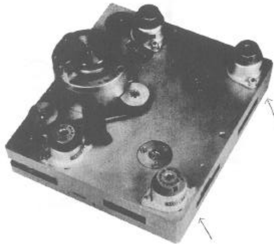
Figure 5 - Vibration Isolators used in the Model CH Recorder
