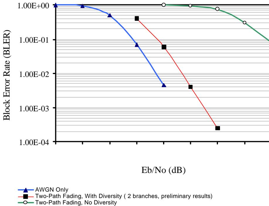
Figure 6) Estimated Block Error Rate (BLER) as a function of available  $E_b/N_0$  (dB) is illustrated with two diversity branches and without diversity for a typical selective fading environment. Numerical values were left blank intentionally as the actual measurements were not completed by the conference paper submission deadline. The actual values will be provided at the conference.
