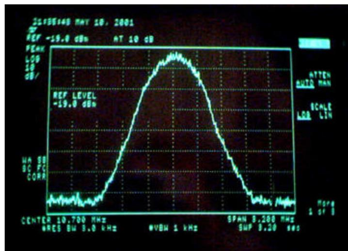
Figure 2) Undistorted spectrum of a 1Mb/s FQPSK
