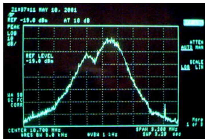
Figure 3) Distorted spectrum of a 1Mb/s FQPSK due to multipath propagation
