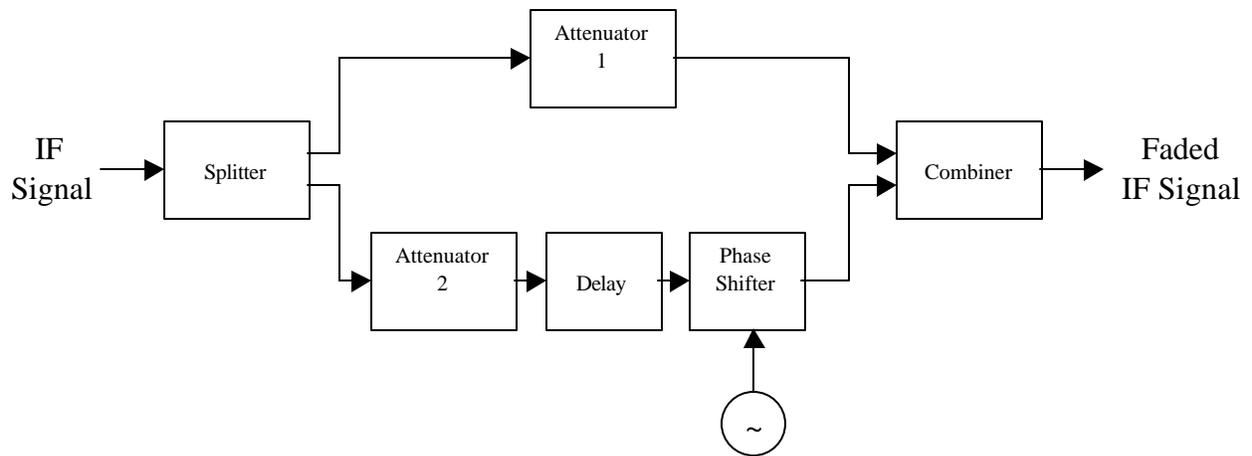
Figure 1) A simple hardware implementation of a two-path fading model
