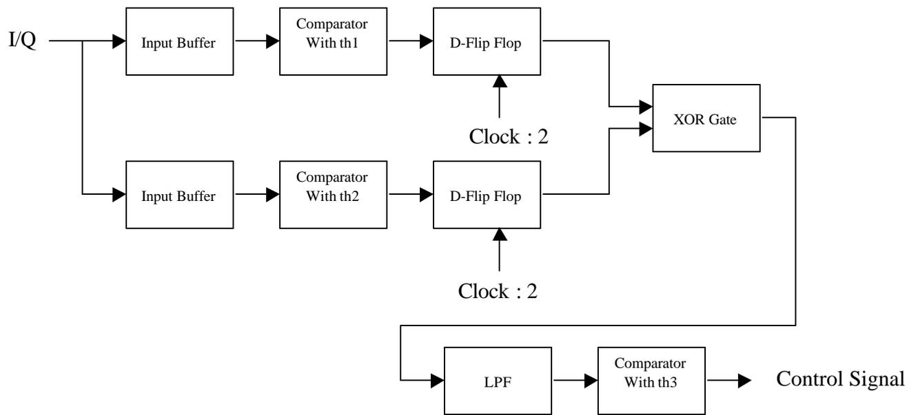
Figure 4) Pseudo-Error Detector Block Diagram
