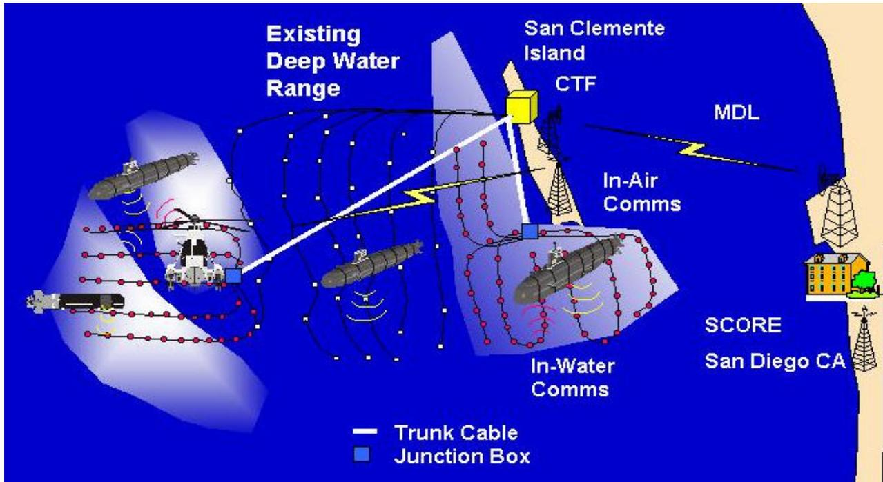
Figure 1 – WC SWUWTR System Configuration
