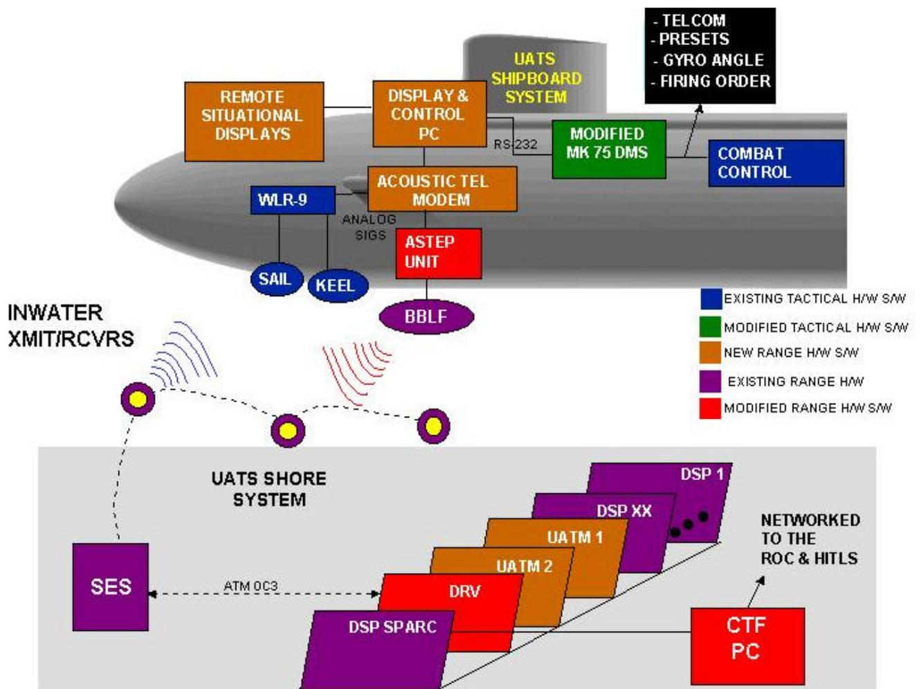
Figure 3 – Underwater Acoustic Telemetry System
