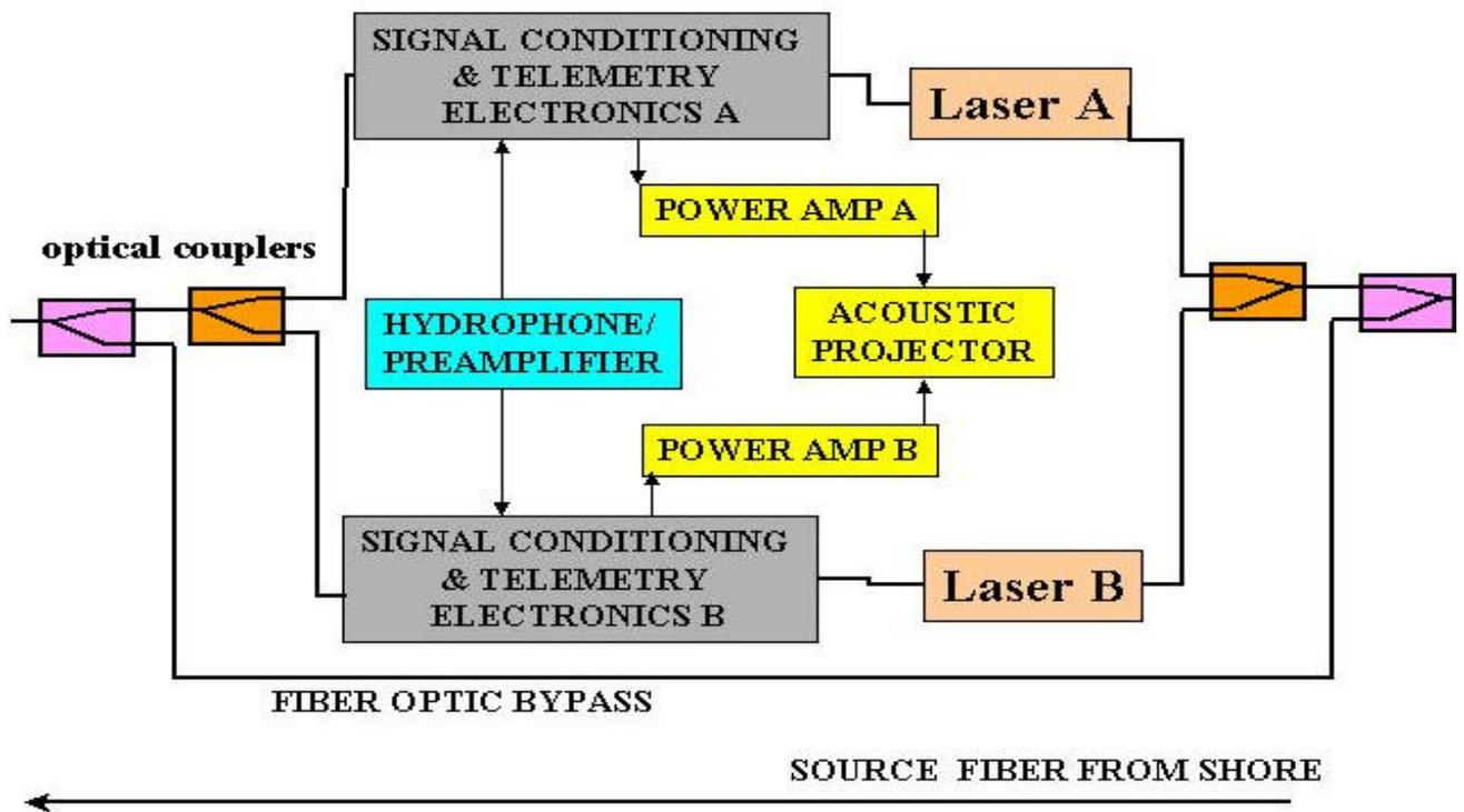
Figure 2 - In-water Electronics Functional Block Diagram
