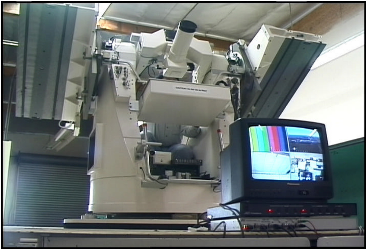
Figure 12 Four channels of real-time video signals are transmitted through embedded FORJ from rotating platform to the control center of the tracker
