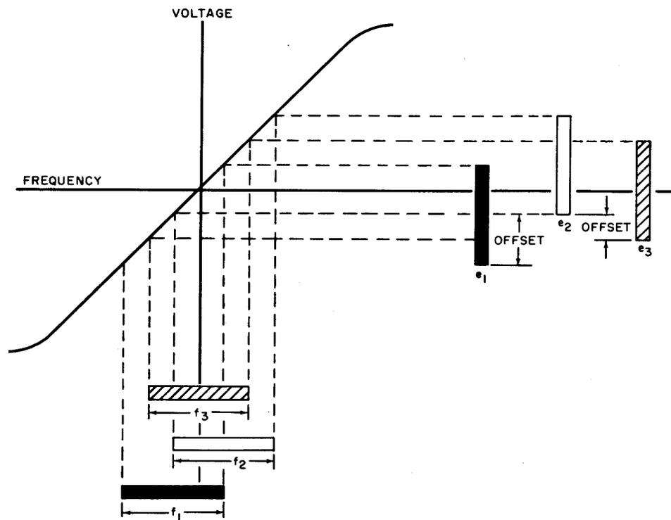
**Figure 9. FM Receiver Discriminator Characteristic Curve**
