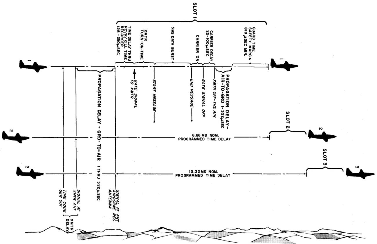
Figure 5. System Data - Flow Time Sequence Chart
