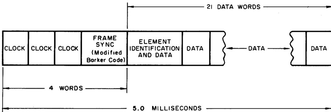
Figure 6. Any Element Data Burst Format
