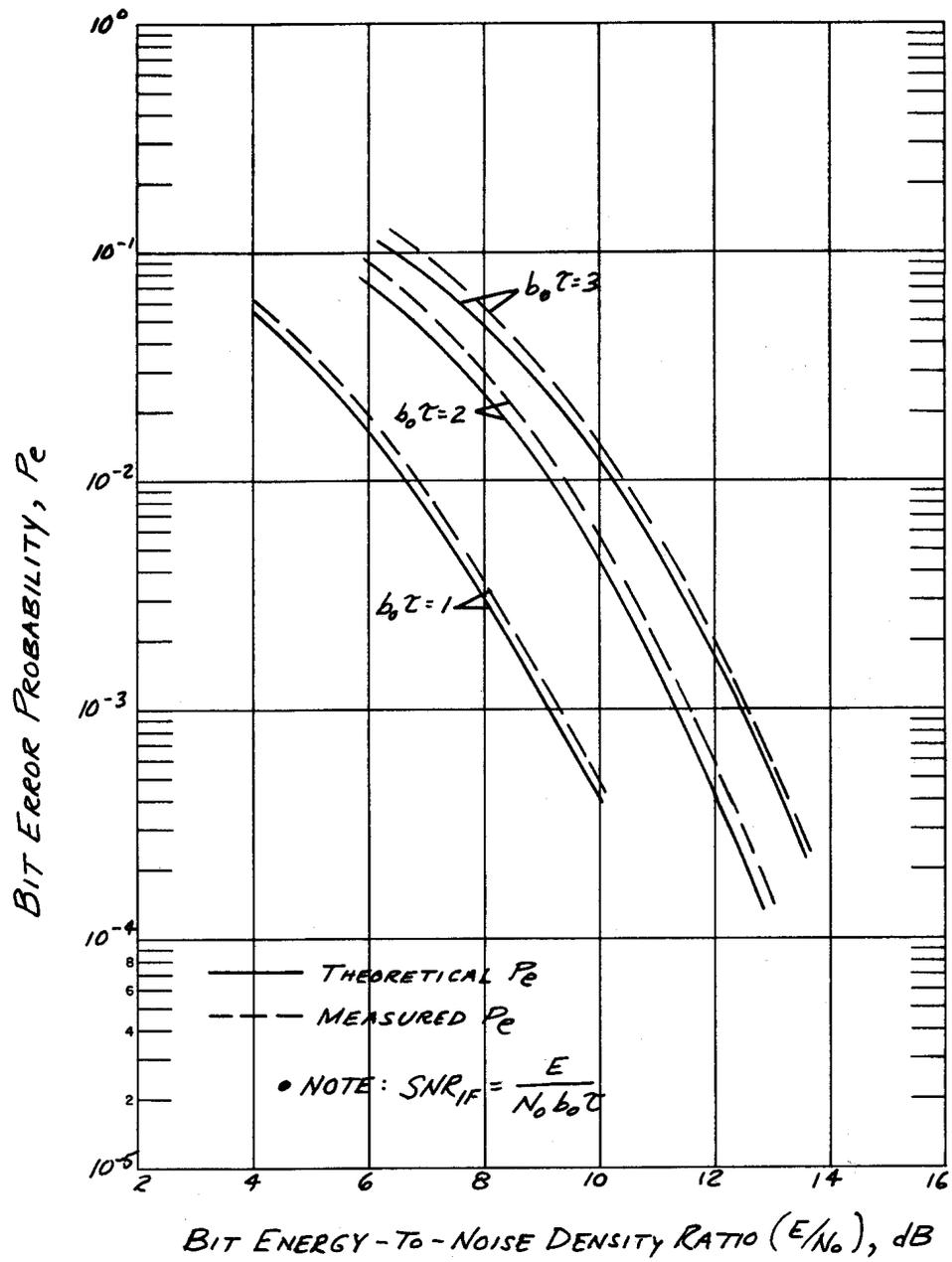
Figure 6. Comparison Of Theoretical And Measured  $P_e$
