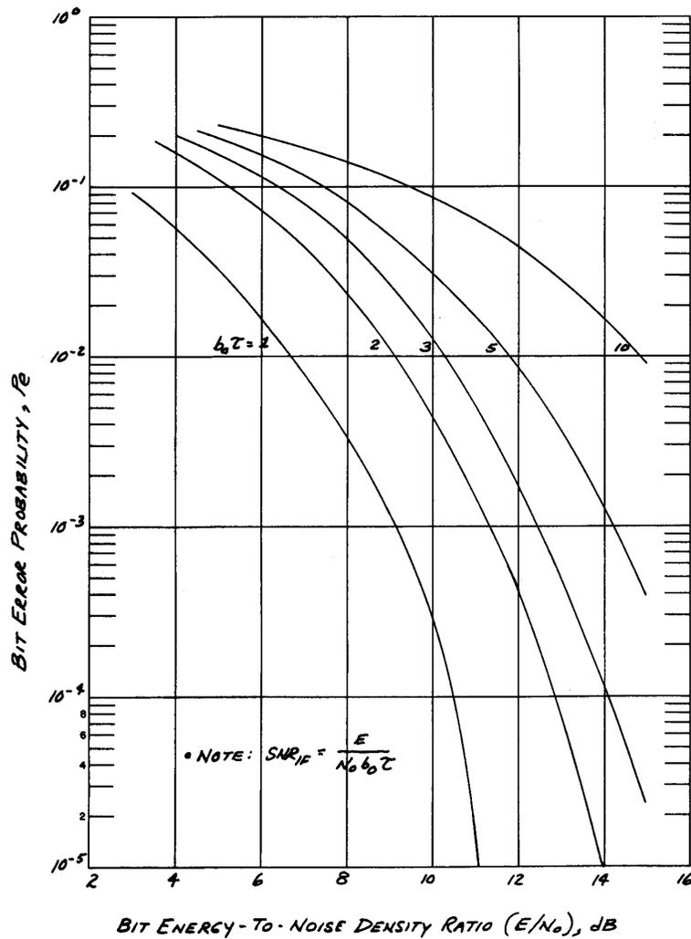
Figure 2.  $P_e$  For Wideband PCM/FM With Discriminator Detection
