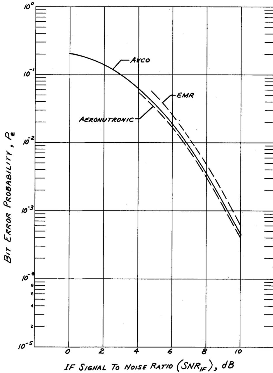
Figure 5. Comparison of Measured  $P_e$  For  $b_o\tau=1$
