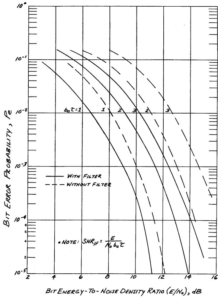
Figure 3.  $P_e$  With And Without Post-Detection Filter
