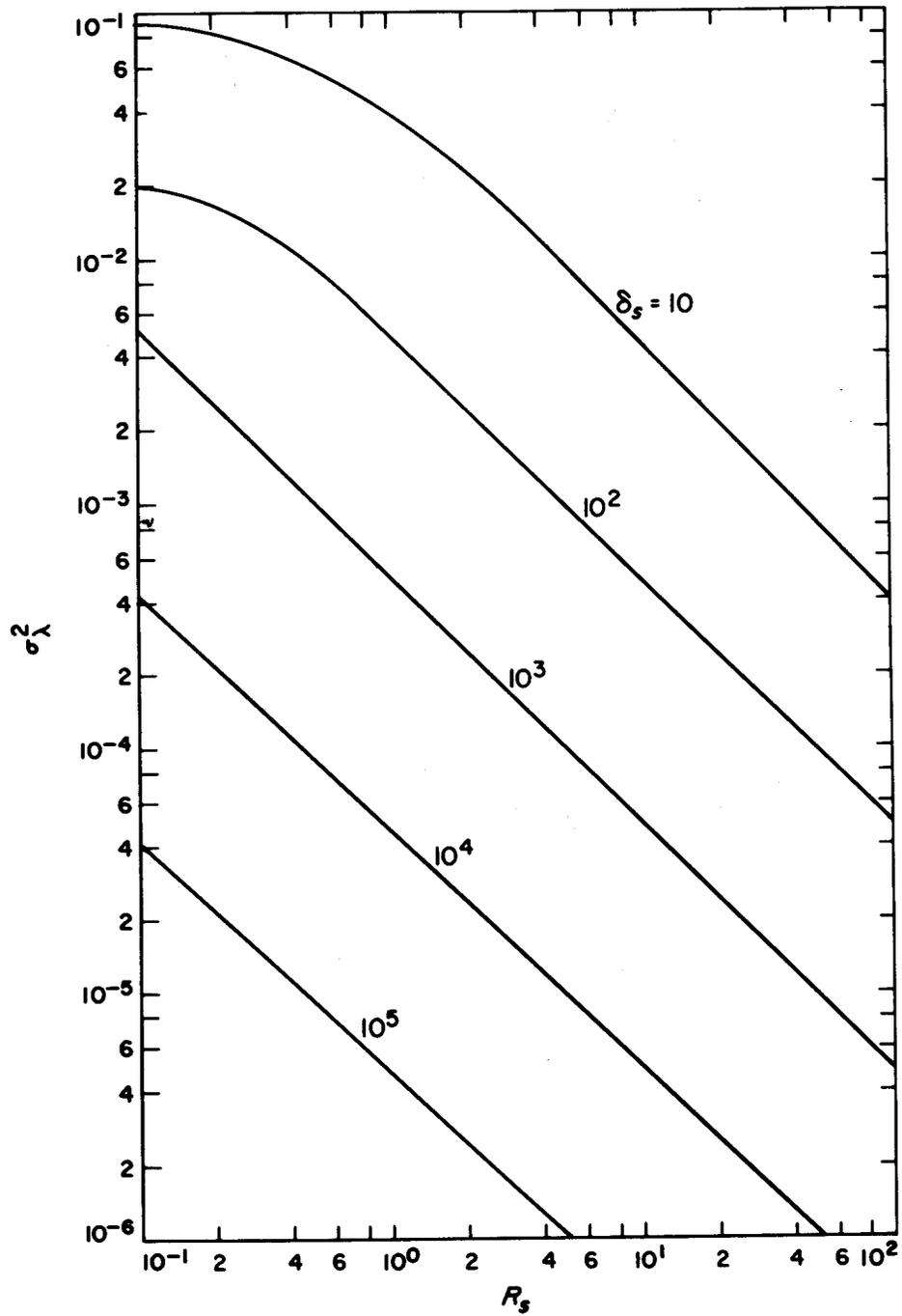
FIG. 4. VARIANCE  $\sigma_\lambda^2$  OF THE NORMALIZED JITTER vs  $R_s$  FOR VARIOUS VALUES OF  $\delta_s$
