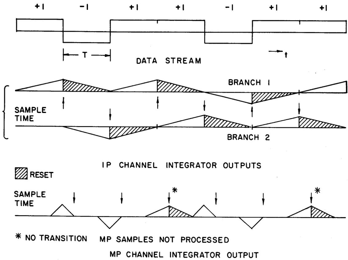
FIG. 7. SYSTEM TIMING CHART FOR  $w = T/2$
