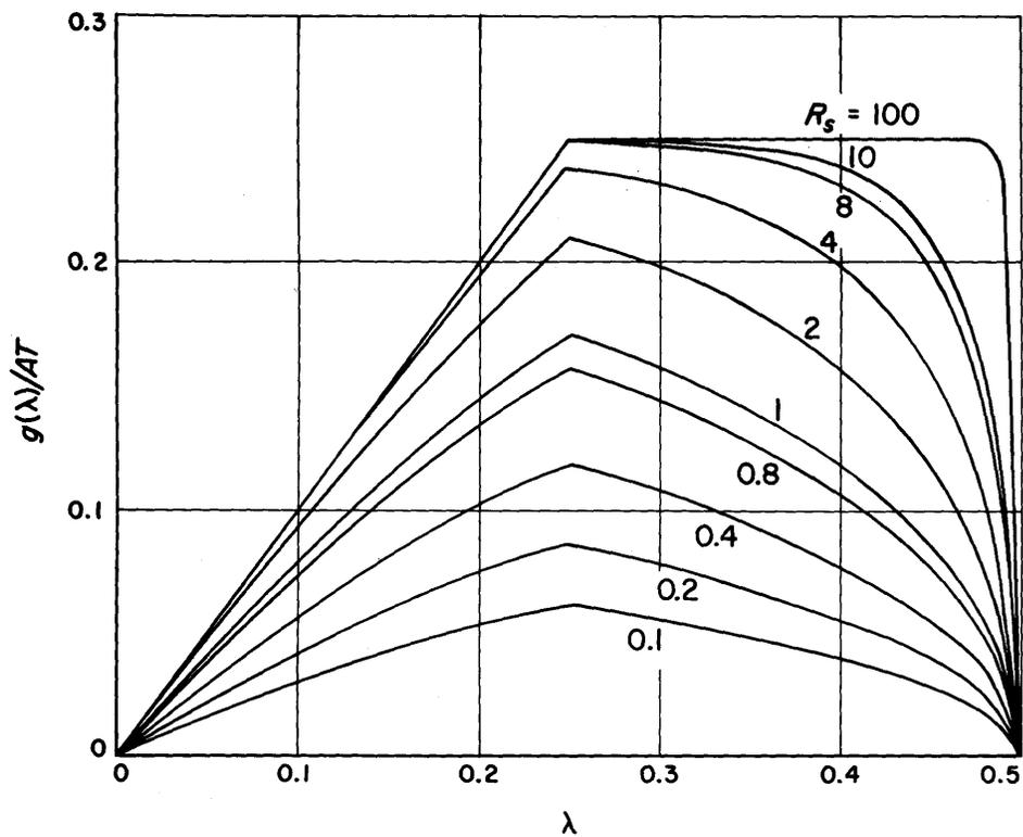
FIG. 5. THE FUNCTION  $g(\lambda)/AT$  vs  $\lambda$  FOR VARIOUS  $R_s$  WITH  $w = T/2$
