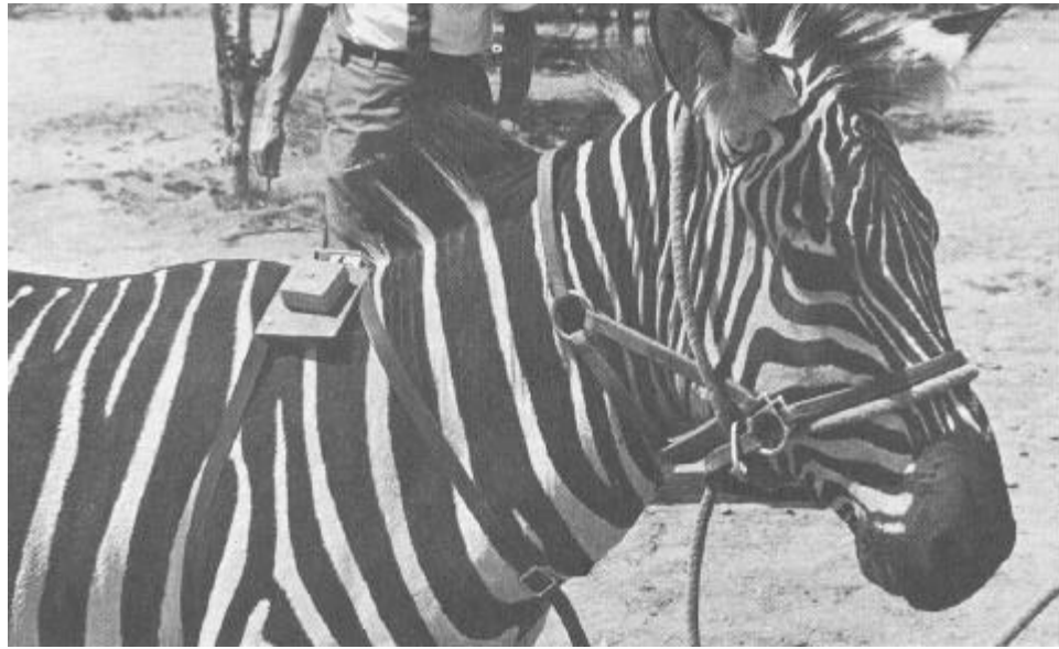
Plate 1A A dual channel telemetry transmitter for the study of skin temperatures in the zebra. This view shows the transmission live antenna mounted on a temporary ground plane surface.
