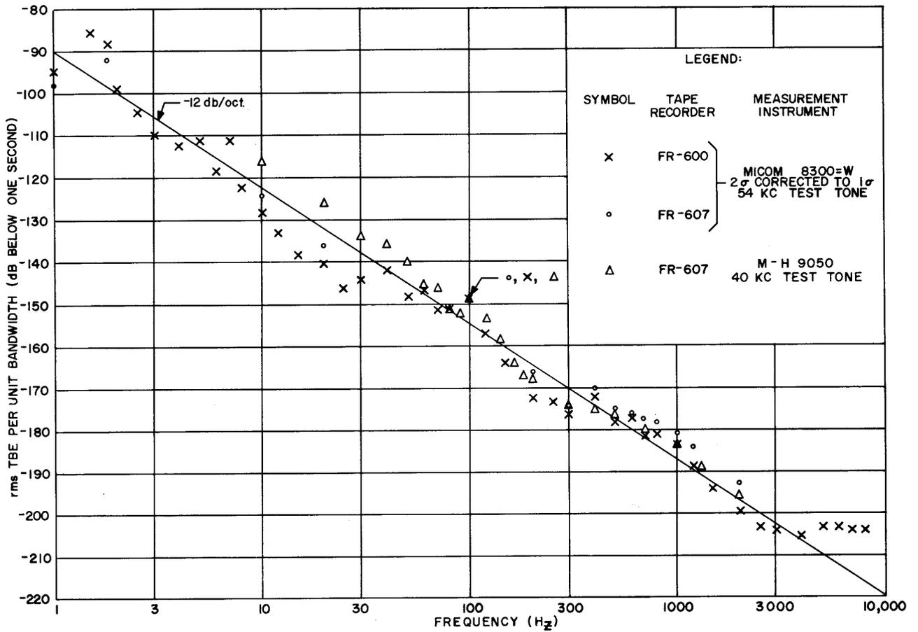
Fig. 1 - Measured Time Base Error Spectrum
