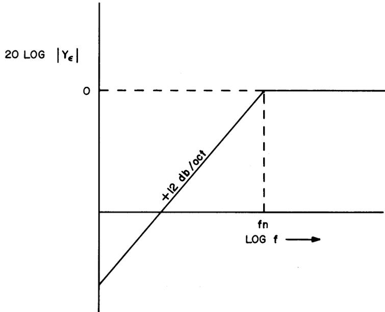
Fig. 2 - Approximate Phase Error Transfer Function
