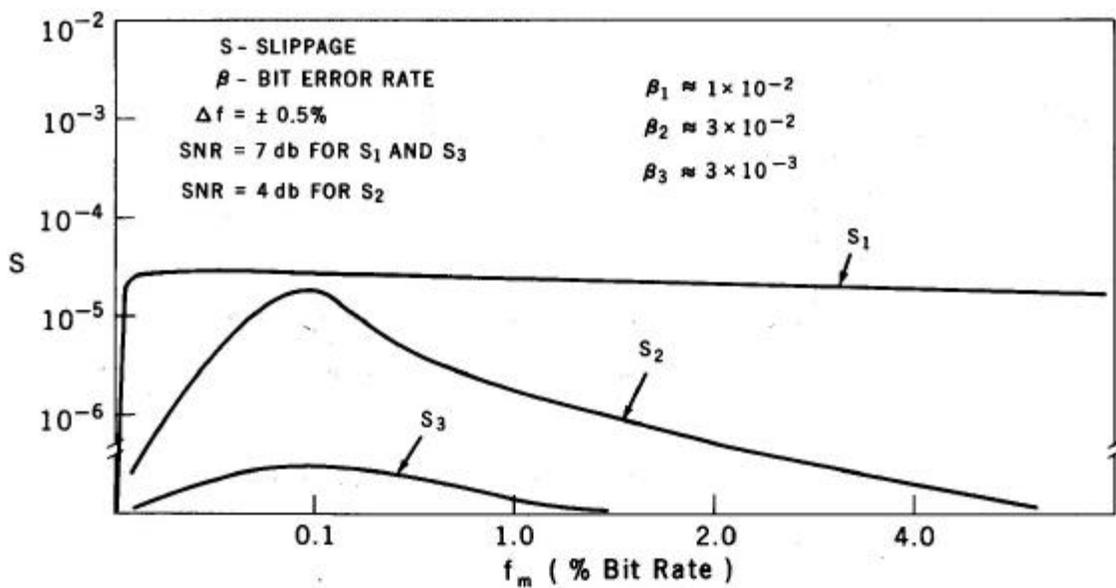
Fig. 7 - Bit Slippage vs.  $f_m$  For  $\Delta f = \pm 0.5\%$
