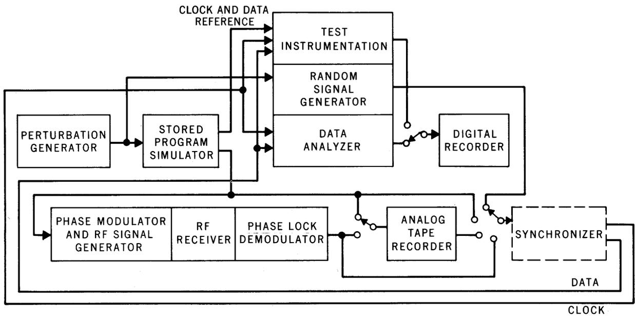
Fig. 9 - PCM BSSC Test Facility.
