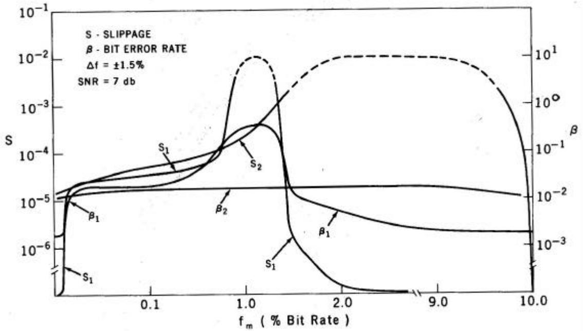
Fig. 7 - Bit Slippage vs.  $f_m$  For  $\Delta f = \pm 1.5\%$
