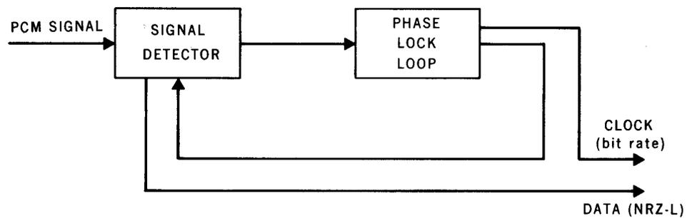
**Fig. 5 - Bit Synchronizer/Signal Conditioner.**
