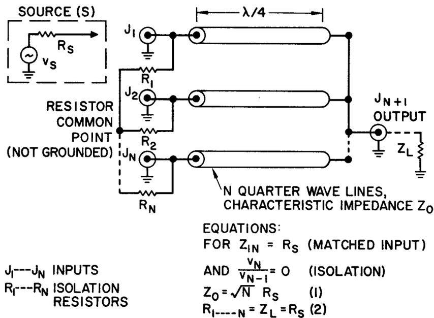
**Figure 1. Schematic and design equations for the basic combiner**
