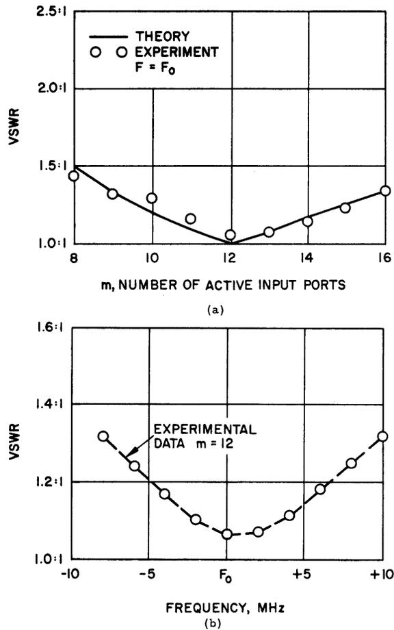
**Figure 2. VSWR versus  $m$  and VSWR versus frequency**
