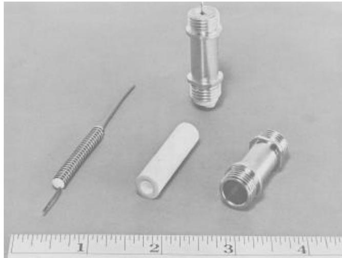
Left to right: Helical center conductor wound on threaded teflon mandrel, teflon sleeve, threaded out tube.
