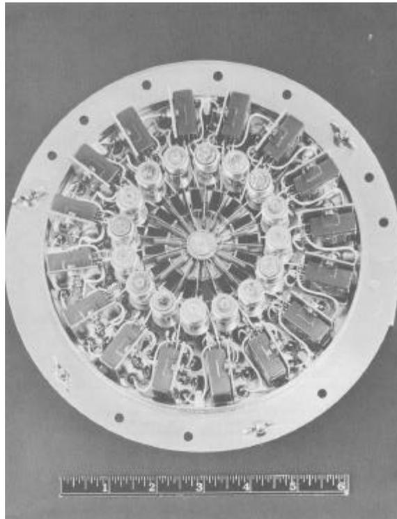
Top view, cover, output connector removed. From inside out: resistor common point, resistors, transmission lines, relays.
