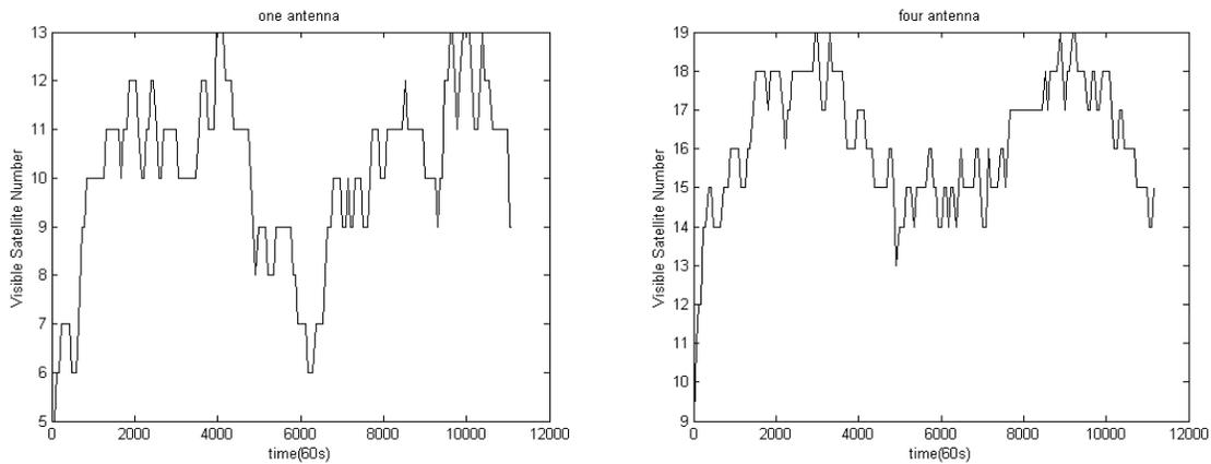
*Figure 1: the number of visible satellite for the high-dynamic spacecraft launching and in-orbital periods under30-MEO Galileo constellations (one and four antenna)*
