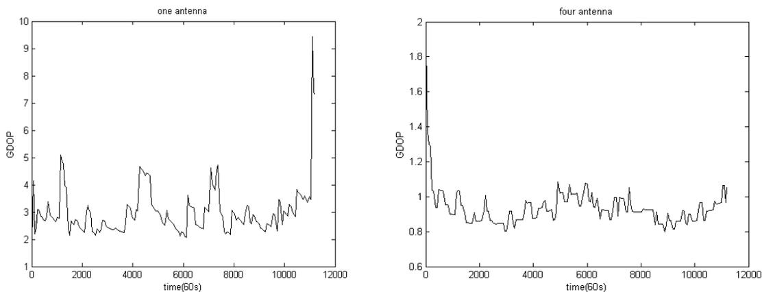
*Figure 2: GDOP values for the high-dynamic spacecraft launching and in-orbital periods under30-MEO Galileo constellations (one and four antenna)*
