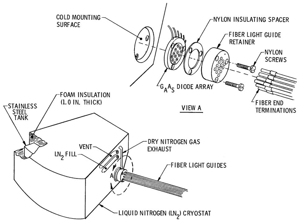
**Figure 5. Relation of Components to Fiber Optic Light Guides and Light Guide Retainer**
