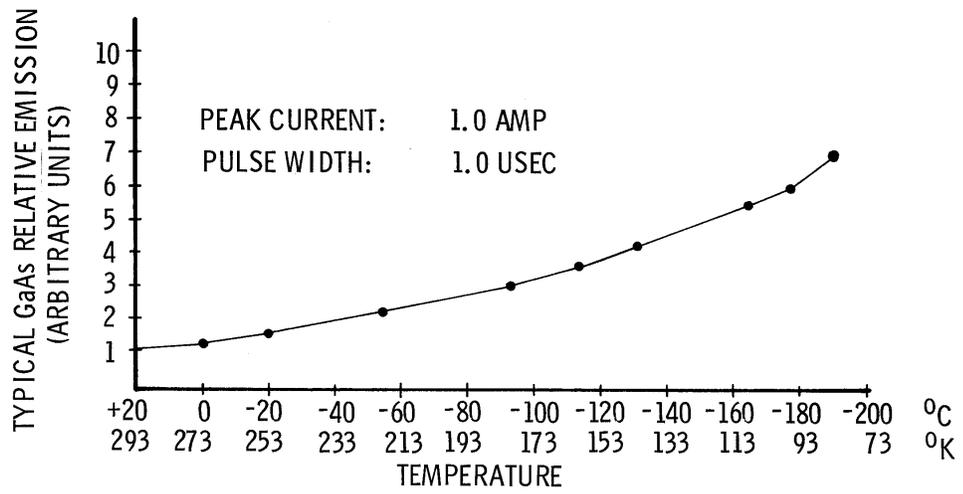
**Figure 3. GaAs Relative Emission vs Temperature**
