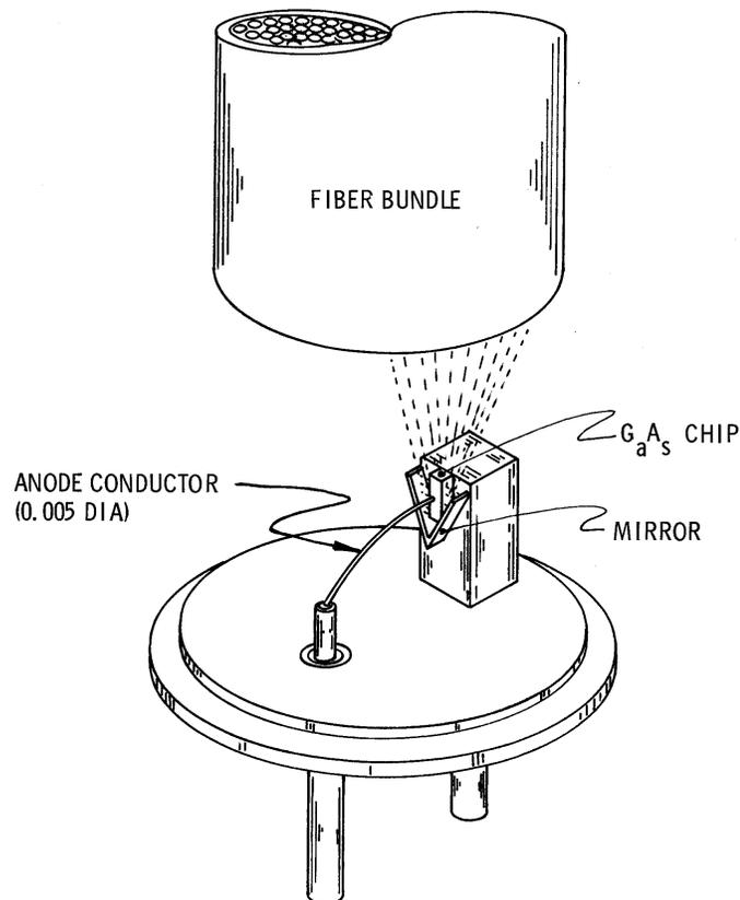
**Figure 6. GaAs Diode Configuration**
