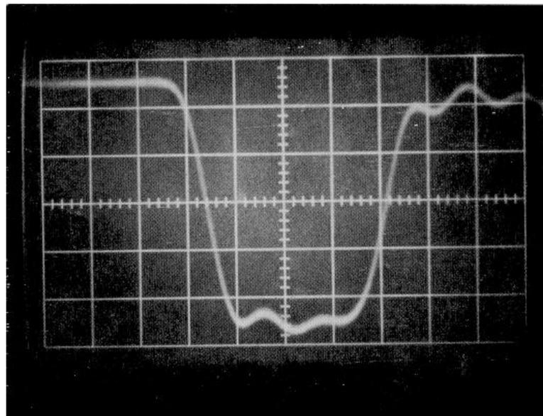
**Figure 8. System Rise Time (Horizontal = 5 nsec/div)**
