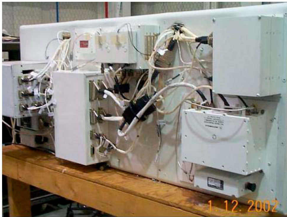
FIGURE 1-1. LDB SUPPORT INSTRUMENTATION PACKAGE WITH THE TDRSS TRANSCEIVER COMMLINK SHOWN.
