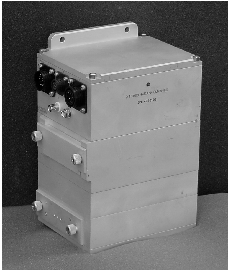
Fig. 2: IVI Data Acquisition System (DAS)
