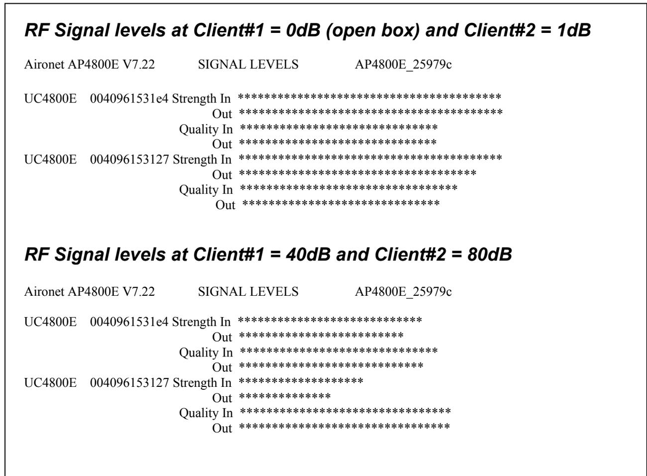
Figure 3 RF Signal strengths for minimal attenuation, top, and more attenuation, bottom
