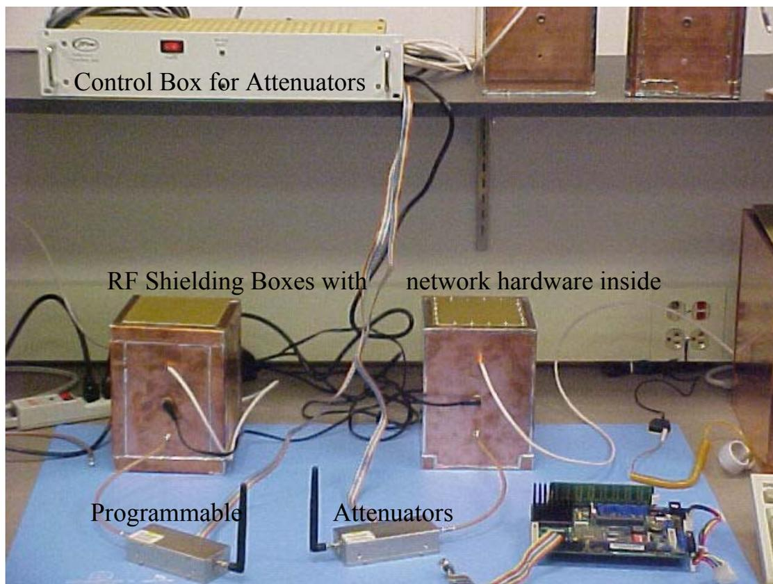
Figure 2 Lab setup with the RF shielding boxes and attenuators [2]
