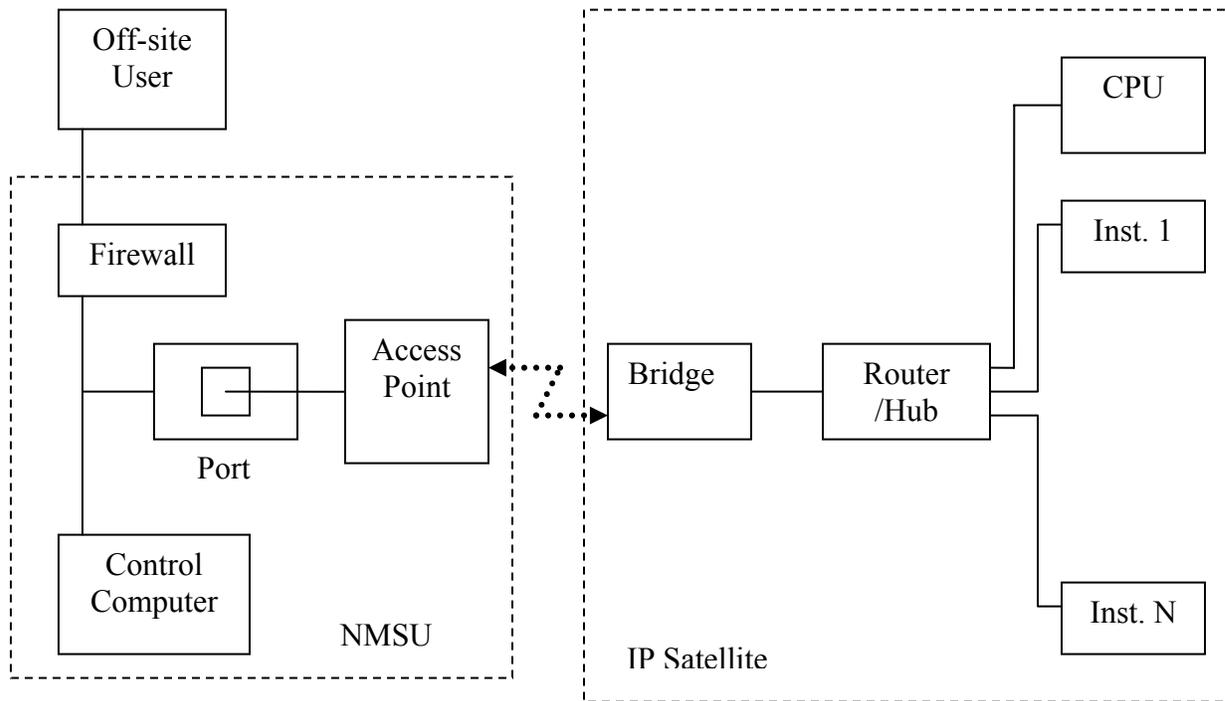
Figure 1 Block diagram of the prototype IP configuration [1]
